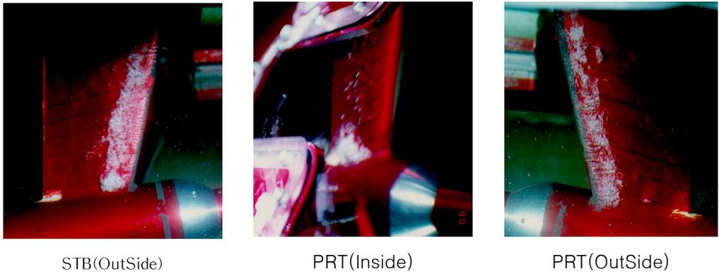
**Fig. 4.19 Cavitation sketch and photographs of the 1st designed strut**
