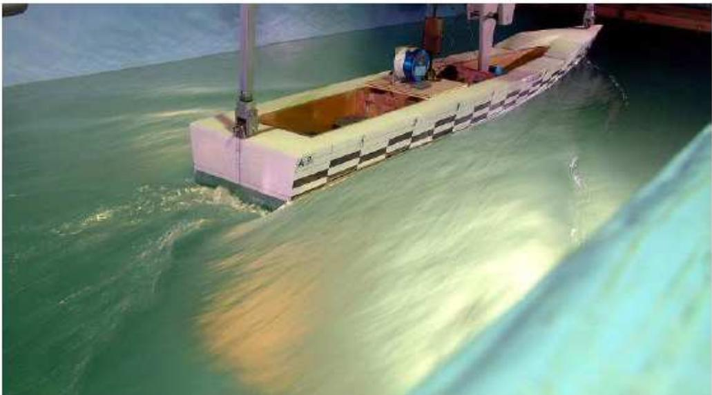
Fig. 5.20 Wave Pattern( $V_s = 15.0$  Knot)
