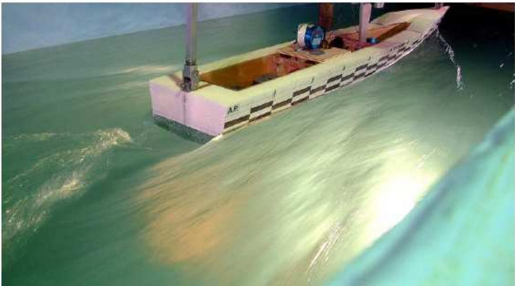
Fig. 5.22 Wave Pattern( $V_s = 20.0$  Knot)
