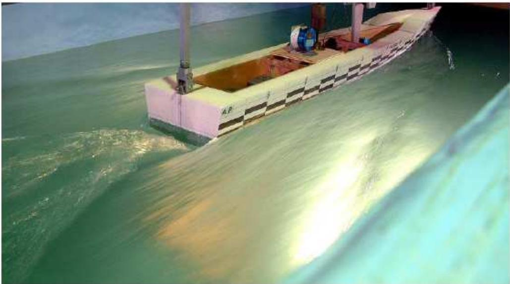
Fig.5.21 Wave Pattern( $V_s = 17.5$  Knot)
