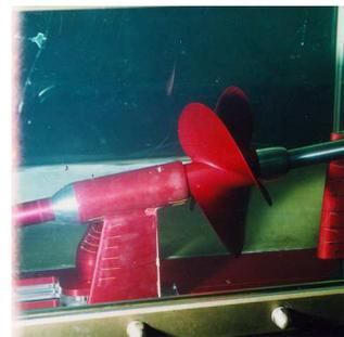
Tuft test(Side View)
