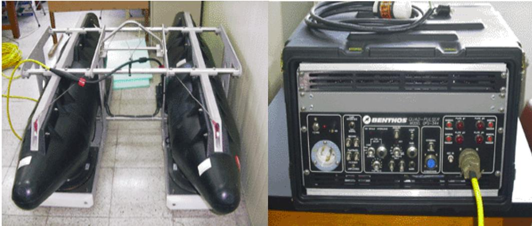
Fig. 1 Boomer system(left : quad-pulser , right : transceiver)
