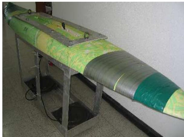
Fig. 5 Shallow marine seismic source
