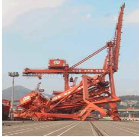
Fig. 3.14 Destruction of Container Cranes at Gammam terminal and Pier No.5
