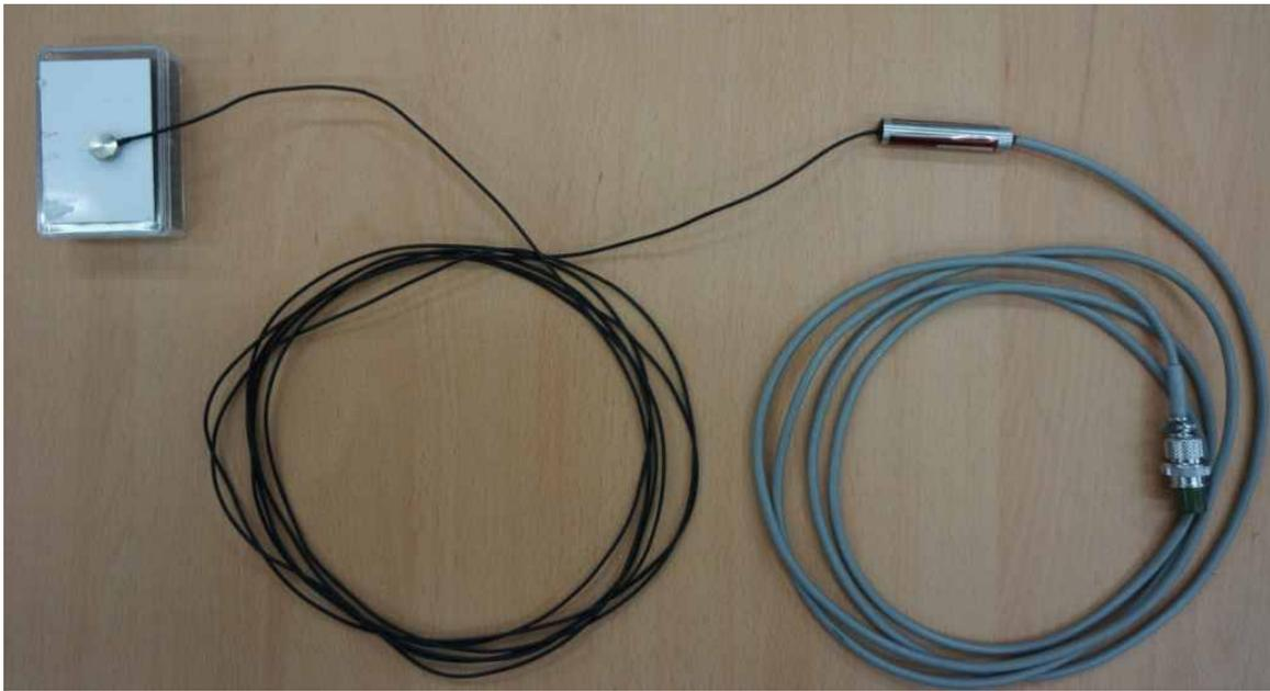
**Figure 6.3** Excess pore pressure Gage for Test of 2-Dimensional Wave Basin
