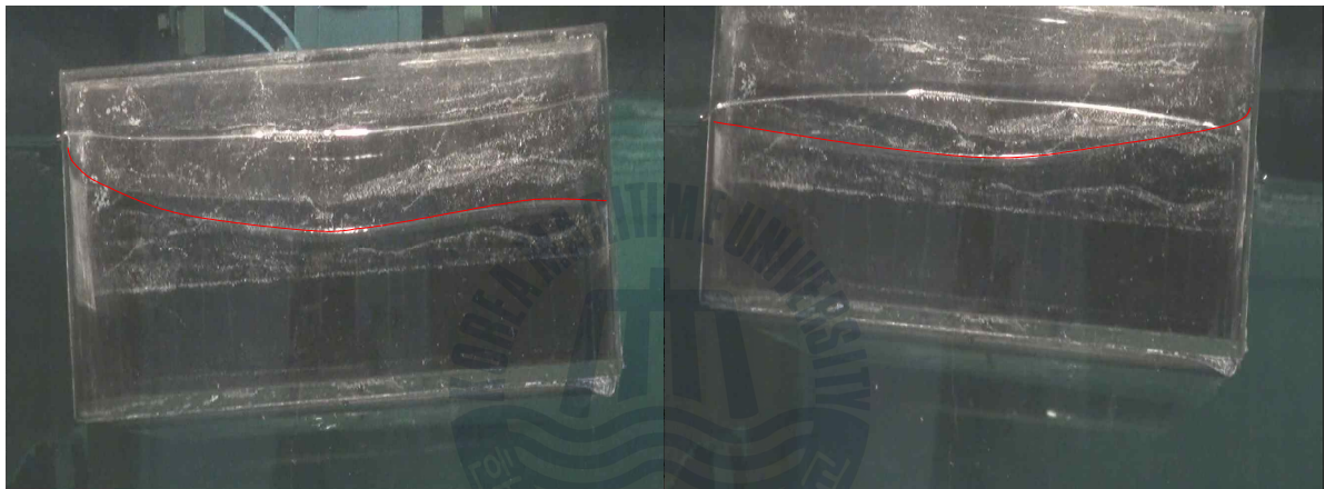
Fig. A.3-2 Incident wave period : 0.8 sec
