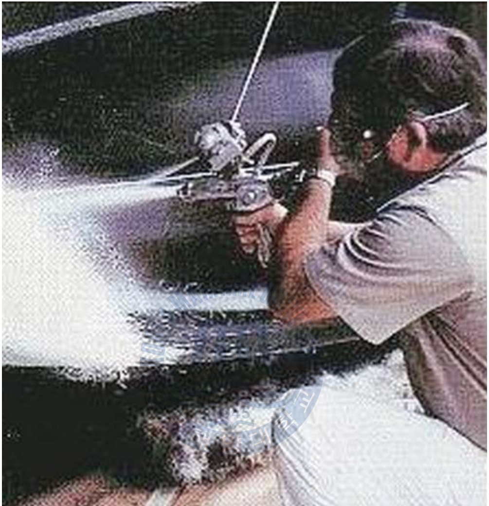
Fig. 2.2 Spray up process
