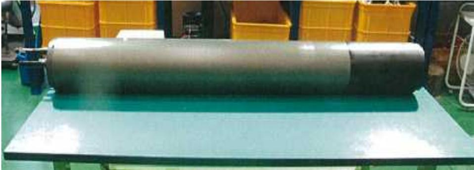
Fig. 39 Hull for Pressure-resistant test
