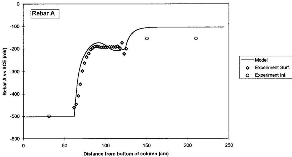
**Figure 3.2:** Potential at the concrete surface along each rebar (Not connected with sacrificial anode) [10]
