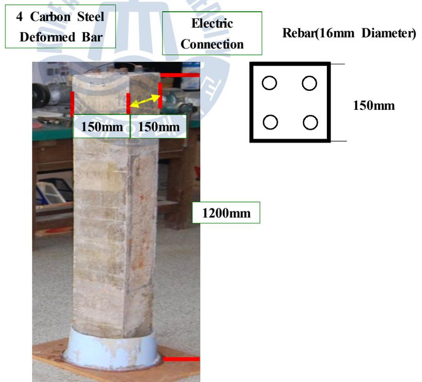
**Figure 4.1:** Beam-type column specimen with dimension
