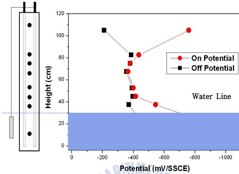
**Figure 5.7:** Potential changes when hybrid CP system was applied (Low tide, Specimen #1)
