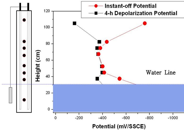
**Figure 5.9:** 4-h Depolarization test of steel in concrete contaminated with chloride. Only the sacrificial anode was disconnected.
