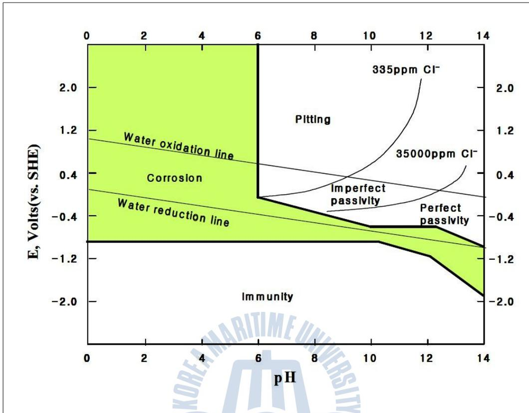
Figure 2.5: E-pH diagram in chloride environment [1]
