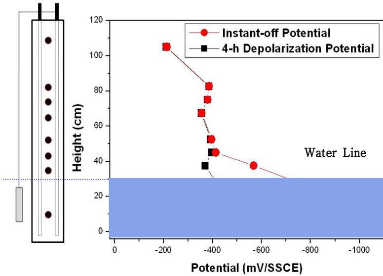
**Figure 5.4:** 4-h depolarization potential of steel with/without SACP (Low tide, Specimen #1, SACP)
