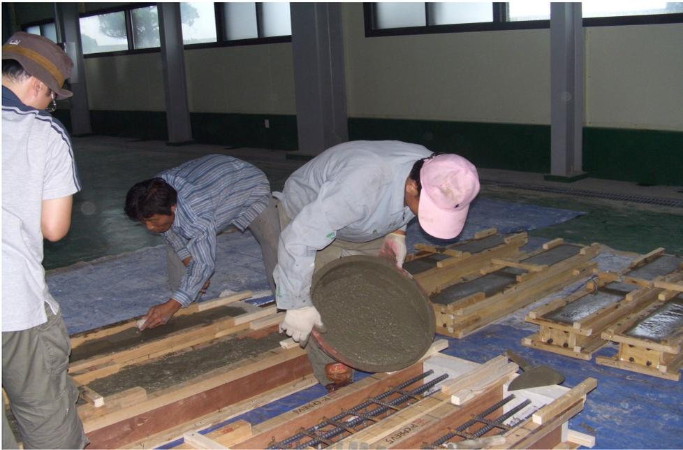
**Figure 4.2:** Manufacturing process of specimens
