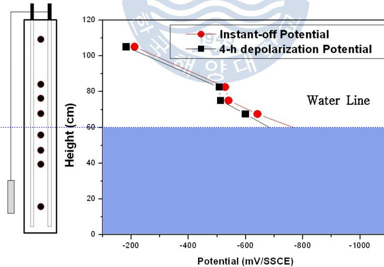
**Figure 5.13:** 4-h depolarization test of steel in concrete contaminated with chloride. Only the sacrificial anode was disconnected.
