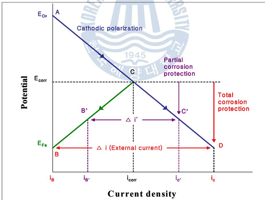
Figure 2.9: Typical polarization curve of ICCP
