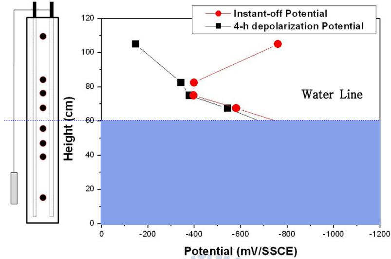
**Figure 5.15:** 4-h depolarization test of steel in concrete contaminated with chloride. Only the anodes were disconnected.
