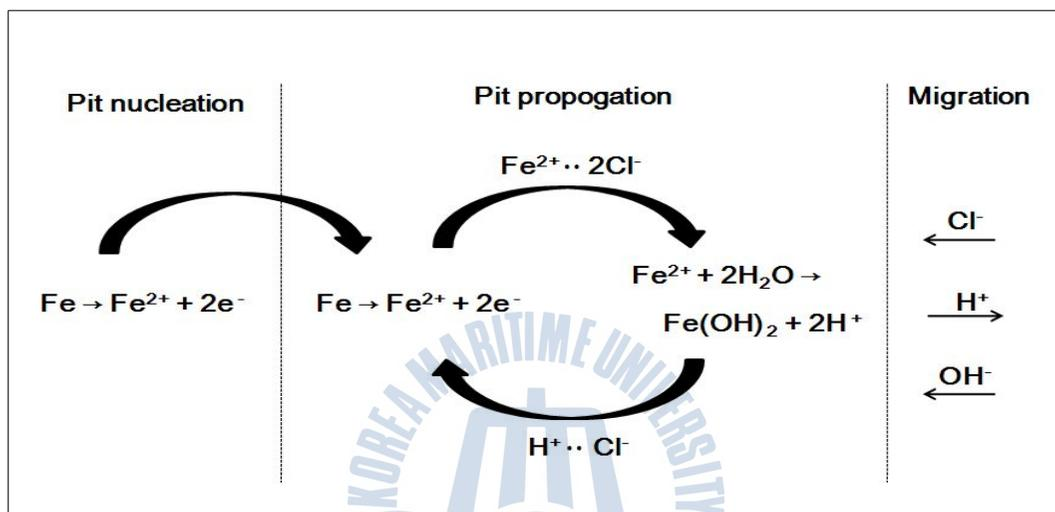
**Figure 2.4:** An illustration of pit-nucleation and pit-propagation processes leading to corrosion damage
