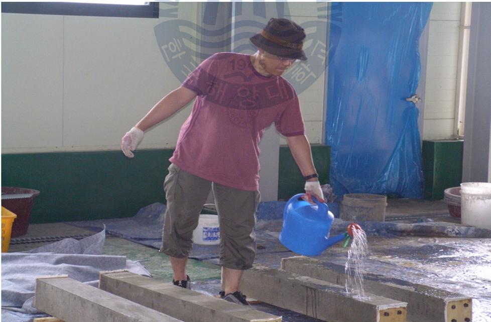
**Figure 4.3:** Curing of specimens
