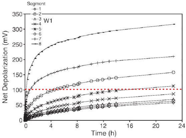
Figure 3.5: Depolarization measured for rebar segment of column [11]
