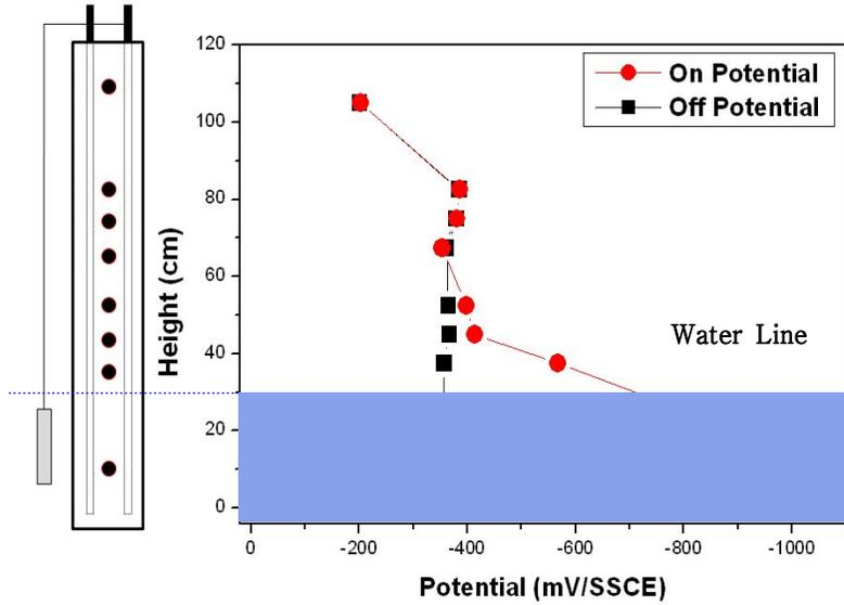
**Figure 5.1:** Potential changes with elevation between CP on & off states (Low tide, Specimen #1)
