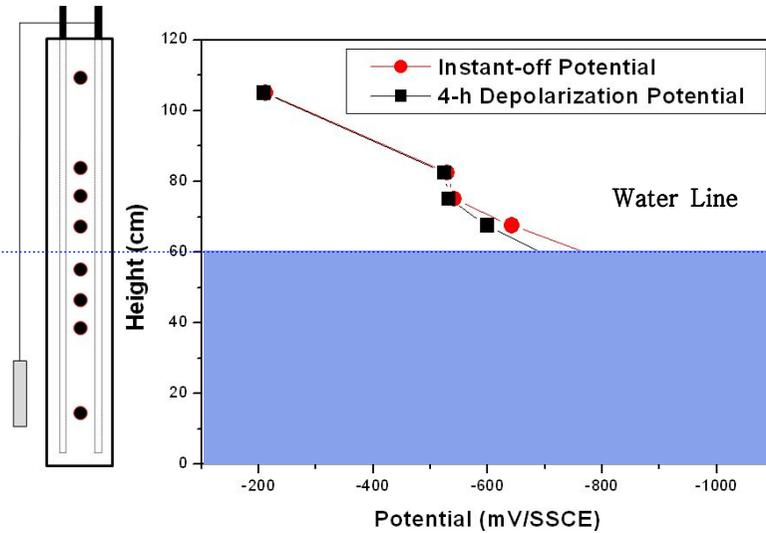
**Figure 5.12:** 4-h depolarization test of steel in concrete contaminated with chloride. Only the sacrificial anode was disconnected.
