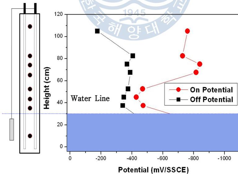
**Figure 5.8:** Potential changes when hybrid CP system was applied (Low tide, Specimen #2)
