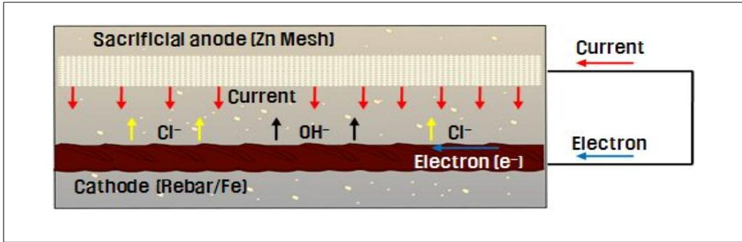
Figure 2.6: Schematic formation of SACP with Zn-mesh
