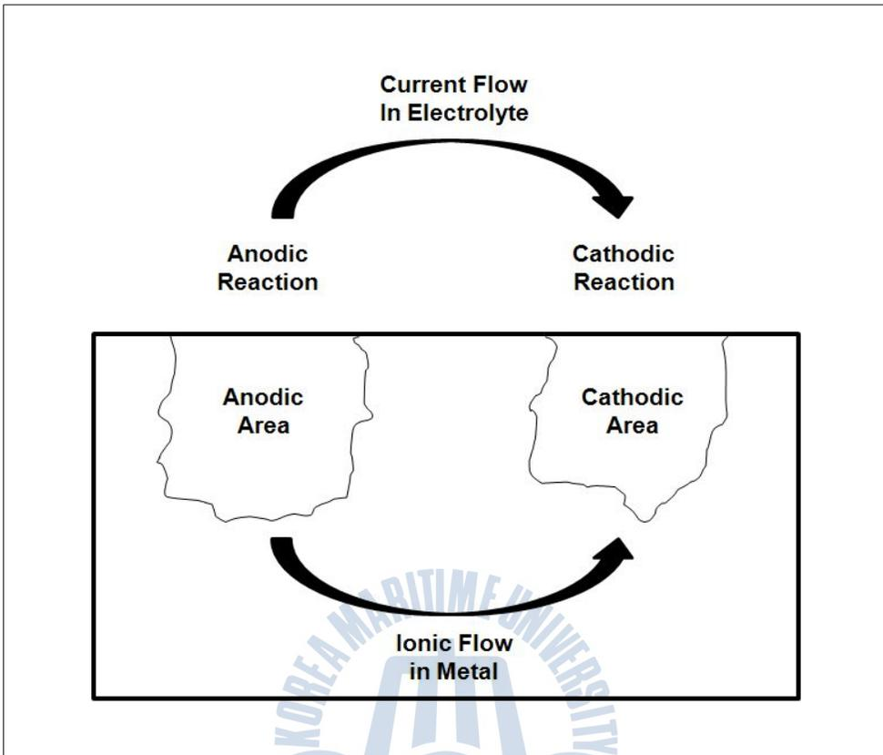
**Figure 2.1:** Electrochemical model of corrosion in metal
