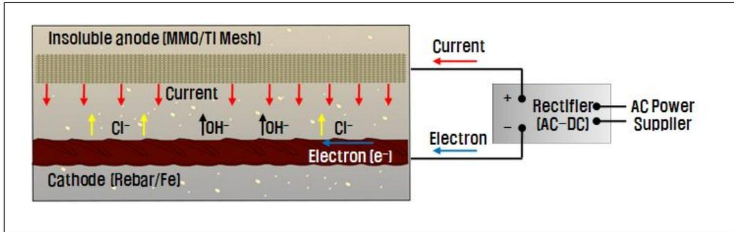
Figure 2.8: Schematic formation of ICCP with MMO/Ti-mesh
