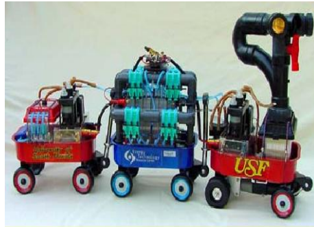
Fig.2.6 “Gastrobot Chew-Chew” - the robot composes a “stomach”, “lung”, gastric pump, “heart” pump, and a six cell MFC stack, Ti plates, carbon electrodes, PEM and E.coli as biocatalyst.
