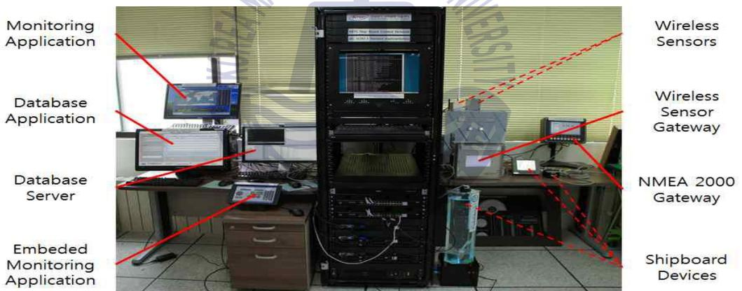
**Fig. 18** Shipboard Integrated Information System
