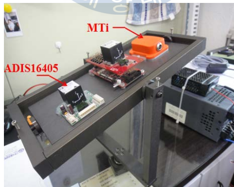
Fig. 4.5 Estimation system on three-axes gimbal structure
