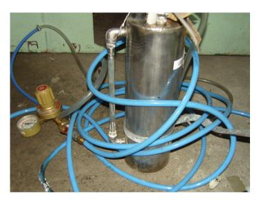
Fig. 15 Photo of 2000ml/min type hydrogen generator
