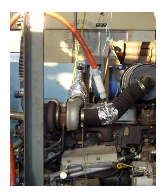
Fig. 14 Connection point of hydrogen generator at intake manifold
