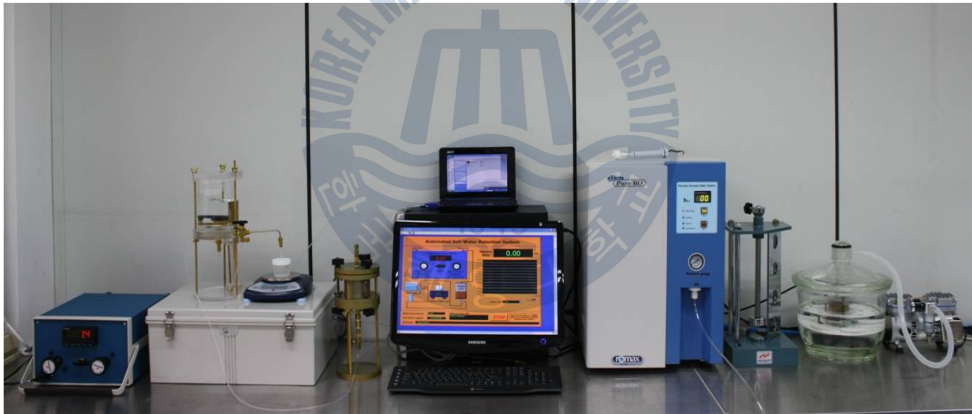
Fig. 3.1 Overall appearance of automated SWCC apparatus (Song et al., 2010)
