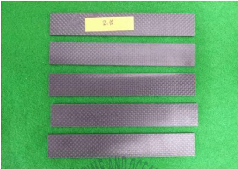
Fig. 3.15 Bending test specimens
