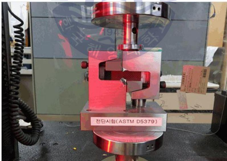
Fig. 3.13 Shear test of composite test specimens
