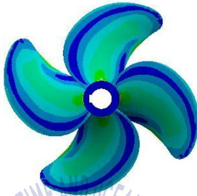
Fig. 5.5 Von-Mises stress - the forward of CFRP propeller
