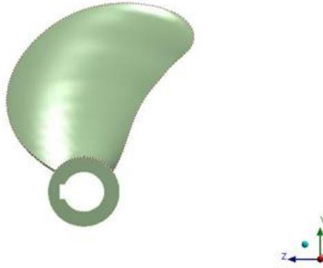
Fig. 5.7 3D model of 1 blade
