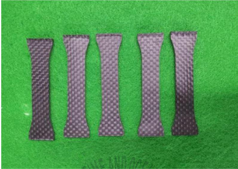
Fig. 3.11 After compression test of composite test specimens
