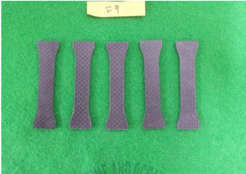
Fig. 3.9 Compression test specimens
