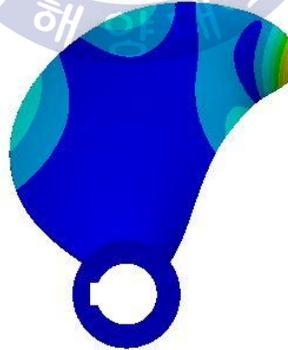
Fig. 5.20 Natural vibration mode of CFRP propeller - 6th mode
