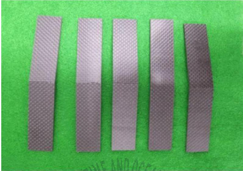
Fig. 3.17 After bending test of composite test specimens
