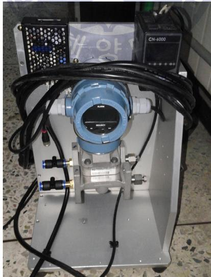
Fig. 2.2 Differential pressure transmitter.
