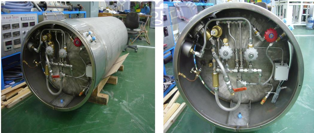
Fig. 3.21 Front piping photo of LNG fuel tank
