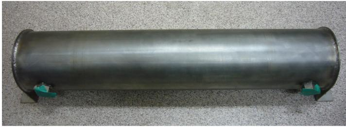
Fig. 3.22 Photo for R134a heat exchanger
