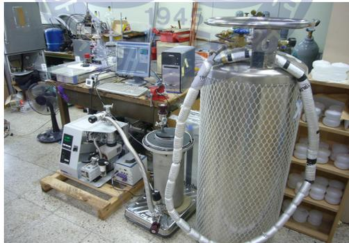
Fig. 3.24 Vacuum pump and LN2 storage tank
