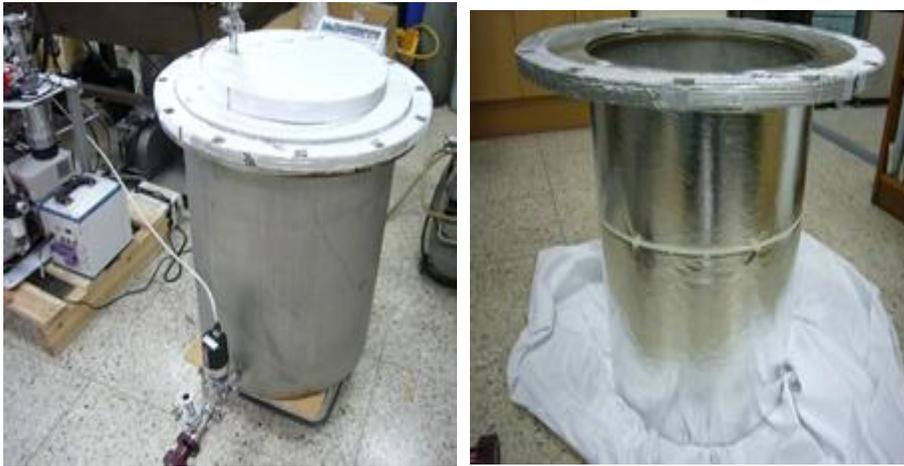
Fig. 3.2 Photos for LN2 cylinder covered with mylar
