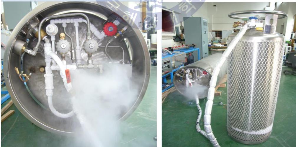
Fig. 4.2 LN2 filling and evaporation rate test
