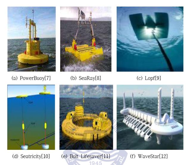
Fig. 1.4 Selected examples of point absorber WECs
