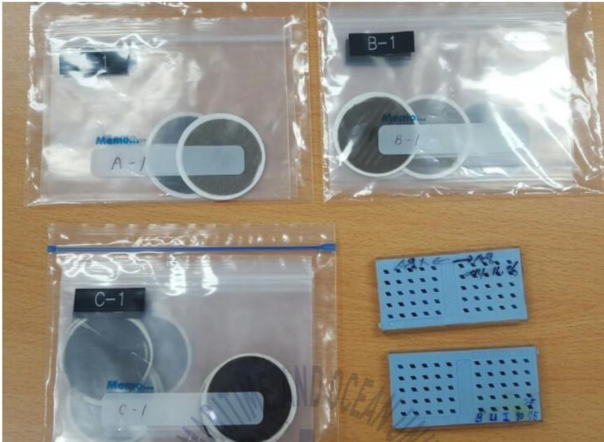
Fig. 2-5 Picture of the soot samples collected from the engines
