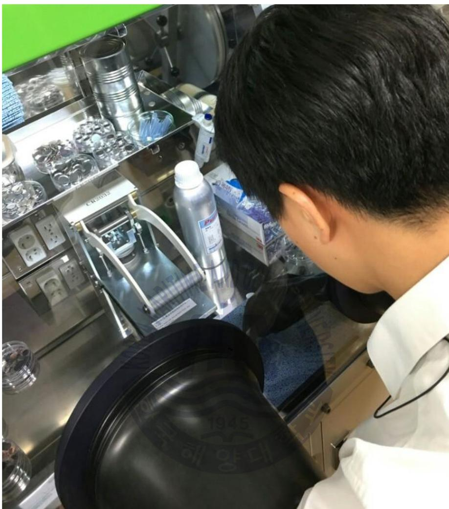
Fig. 2-16 Assembly of a coin cell in the glove box
