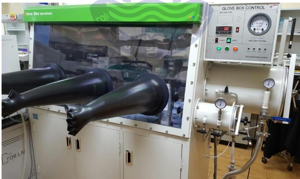
Fig. 2-15 Glove box charged with argon gas
