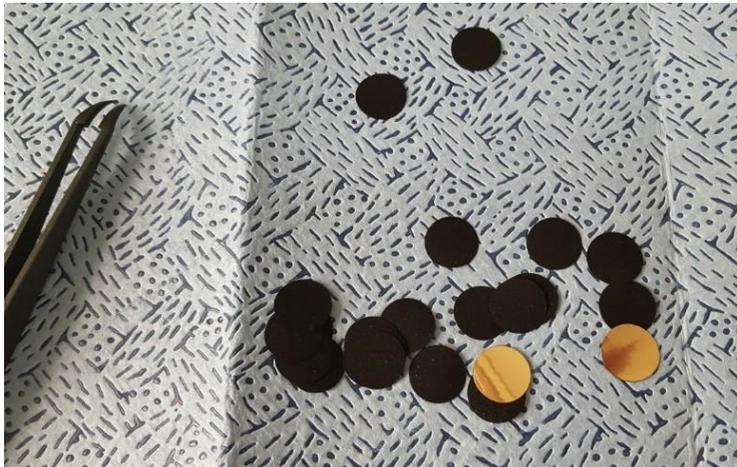
Fig. 2-13 Punched anodes
