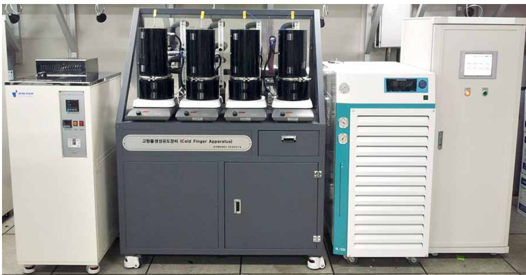
Fig. 10 Front view of the cold finger apparatus(Jung et al., 2014)
