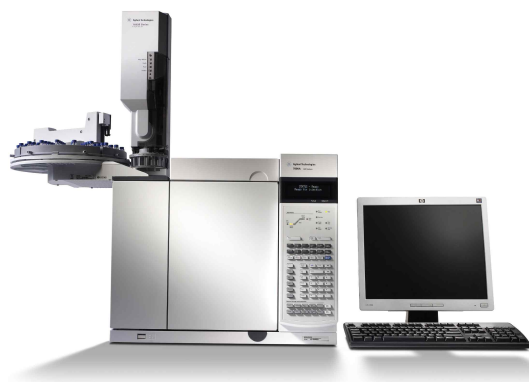
Fig. 6 Gas chromatography for measuring the oil composition
