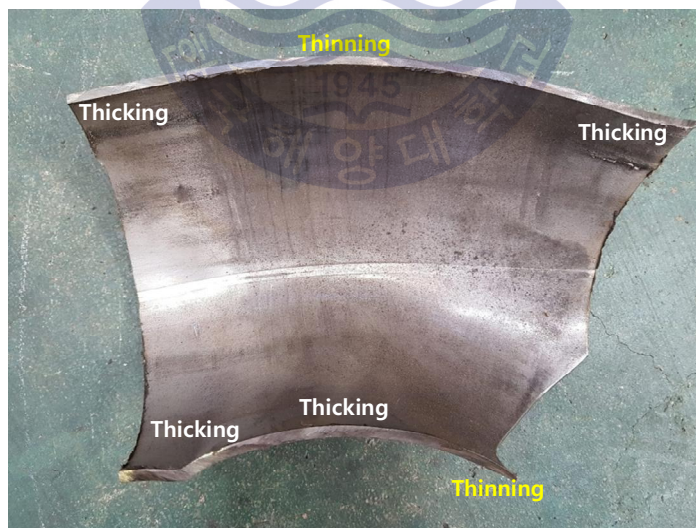
Fig. 29 Variation of elbow thickness
