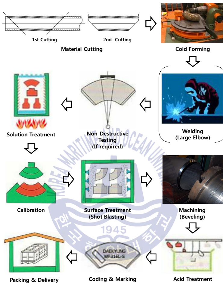
Fig. 1 Conventional manufacturing process for elbow
