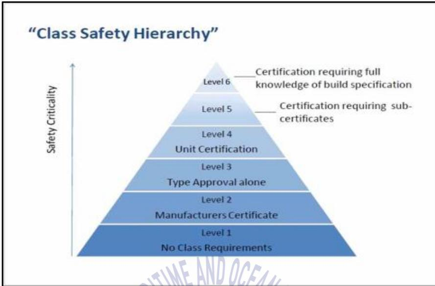
Fig. 6 Pyramid of safety hierarchy for ship equipment(EU MR Group, 2012)
