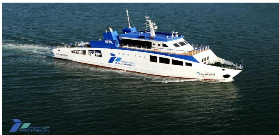
Fig. 1-10 Asia's first LNG fuel vessel "Eco-nuri"
