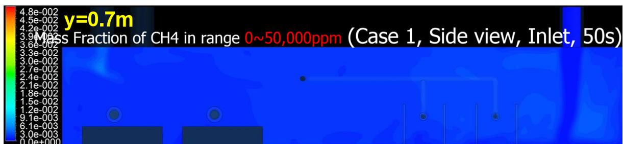
Fig. 4-28 Methane concentrations for case 1 at 50s in the vertical plan of  $y=0.7$  respectively
