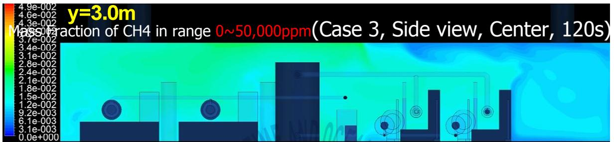
Fig. 4-45 Methane concentrations for case 3 at 120s in the vertical plan of  $y=3.0$  respectively
