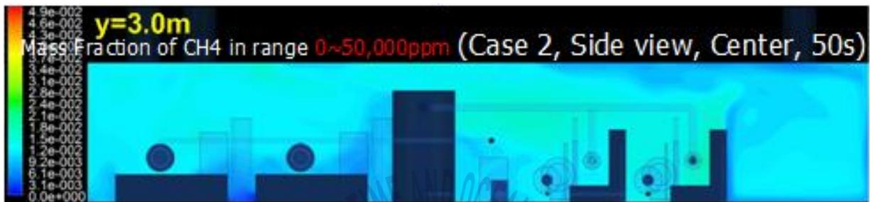
Fig. 4-37 Methane concentrations for case 2 at 50s in the vertical plan of  $y=3.0$  respectively
