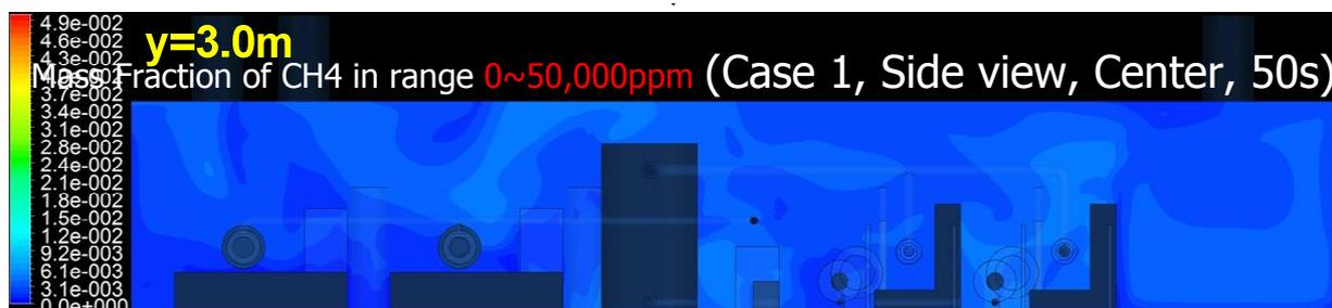
Fig. 4-31 Methane concentrations for case 1 at 50s in the vertical plan of  $y=3.0$ , respectively
