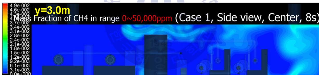
Fig. 4-30 Methane concentrations for case 1 at 8s in the vertical plan of  $y=3.0$ , respectively
