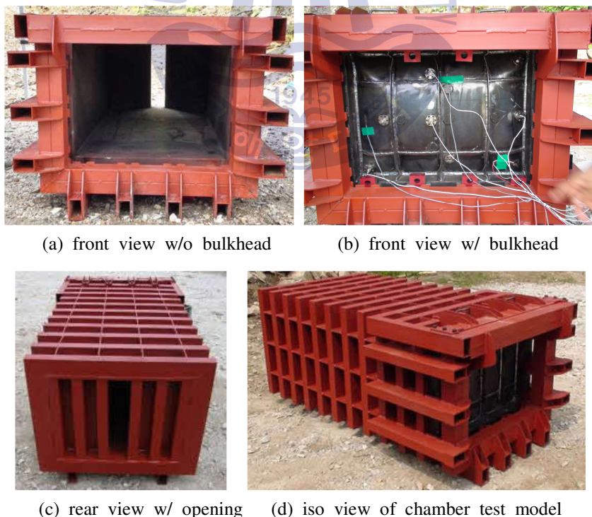
Fig. 6 Reduced scale chamber model for internal blast
