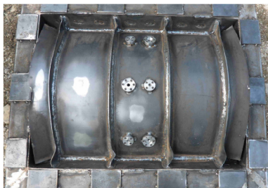
Fig. 10 Damage configurations of reduced scale chamber bulkhead models under internal blast test
