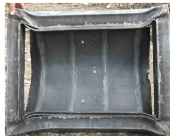
Fig. 10 Damage configurations of reduced scale chamber bulkhead models under internal blast test
