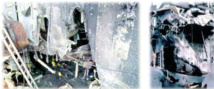
Fig. 2 Internal explosion damage of USS Stark (FFG-31) by Exocet Missiles (Raymond, 2001)
