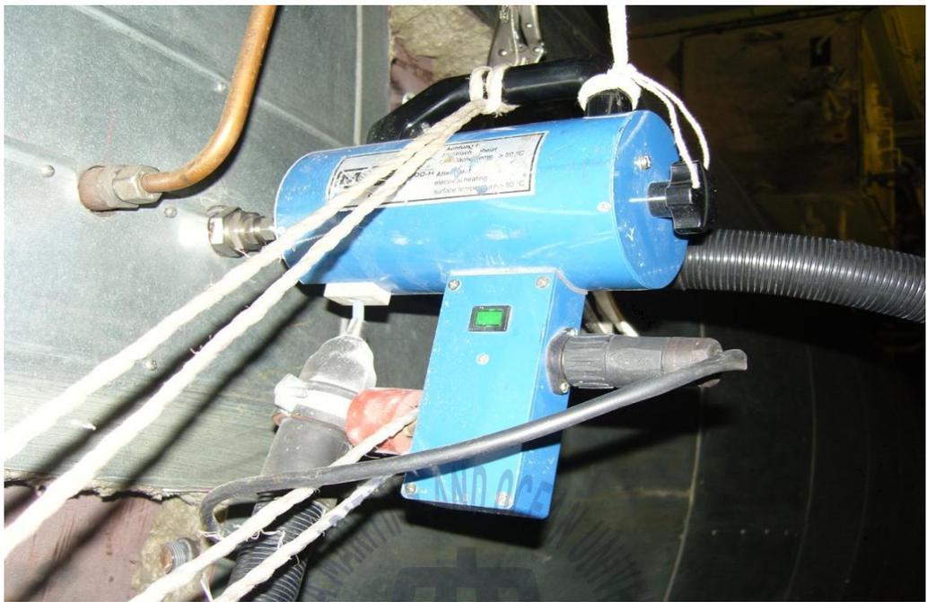
Fig. 3.2.1 NOx and smoke measurement at exhaust gas line
