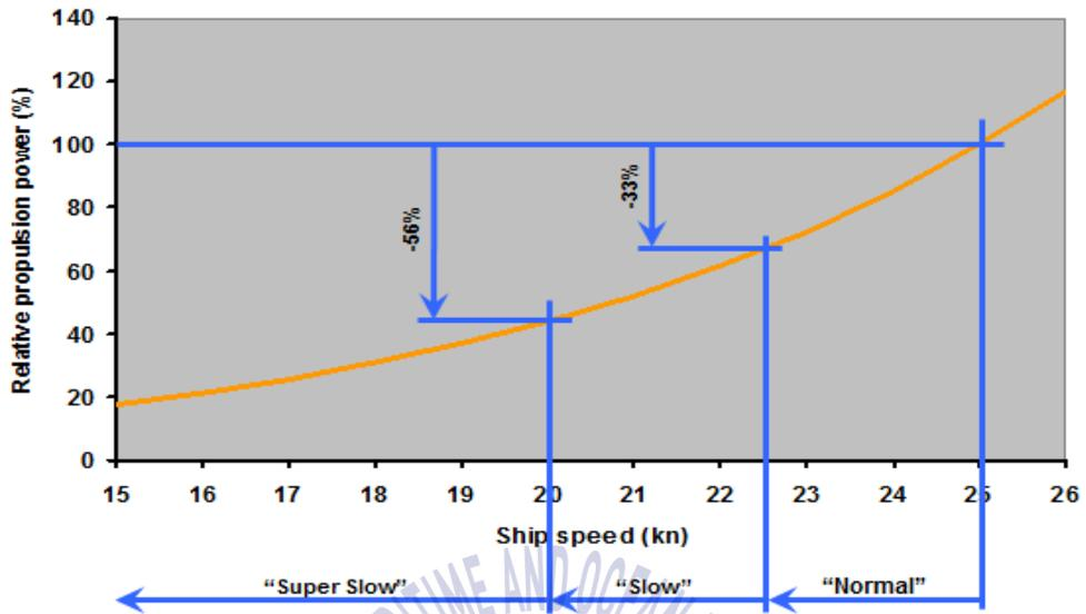
Fig. 3.3.1 Relation between ship speed and propulsion power
