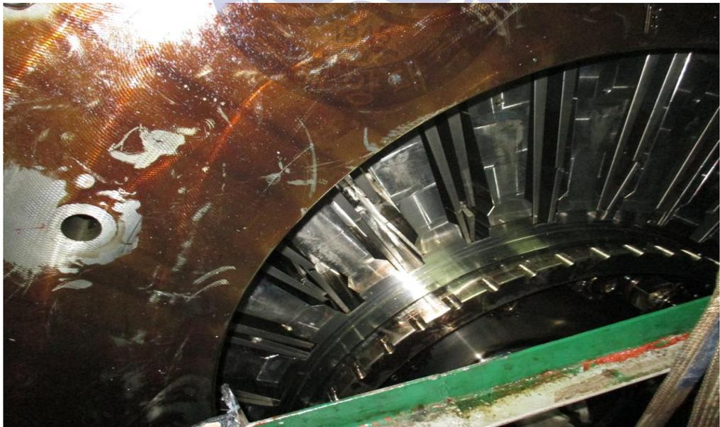
Fig. 3.3.12 Broken damper inside for 5RT-flex58T-D (YZ-6)
