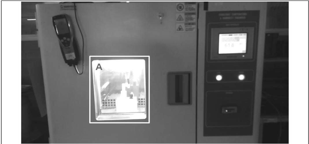
(a) Sensor installation of temperature and humidity chamber
