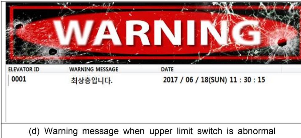
**Fig. 78** Output screen according to upper limit switch test
