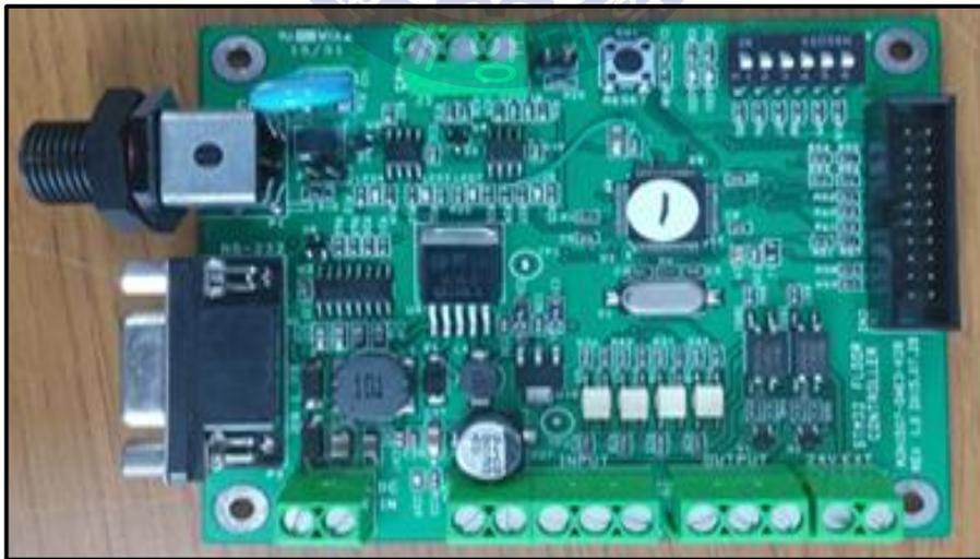
Fig. 40 Floor controller PCB
