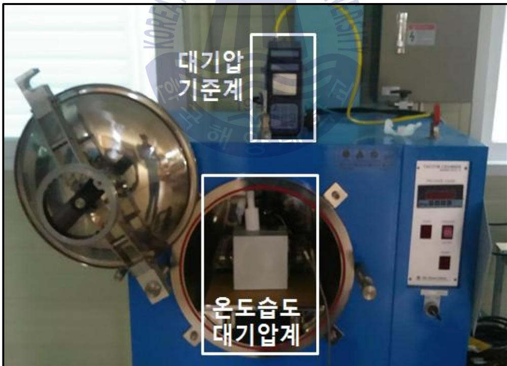
Fig. 66 Atmospheric pressure chamber sensor installation
