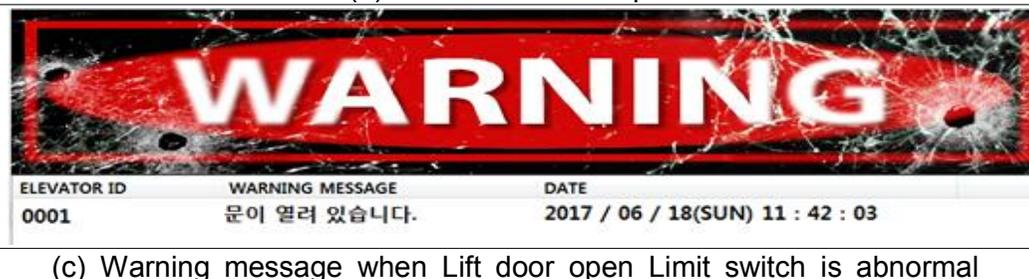
(c) Warning message when Lift door open Limit switch is abnormal
