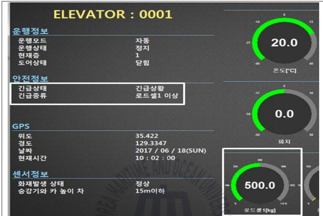
(a) The value of load cell 1 : 500Kg
