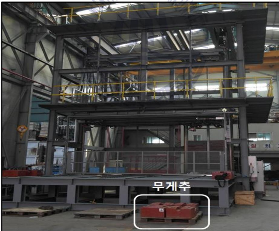
**Fig. 74** Load cell weight measurement test
