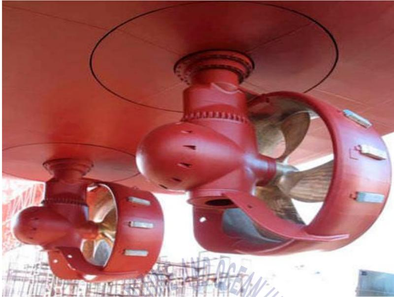
Fig. 2.7 Azimuth Thruster
