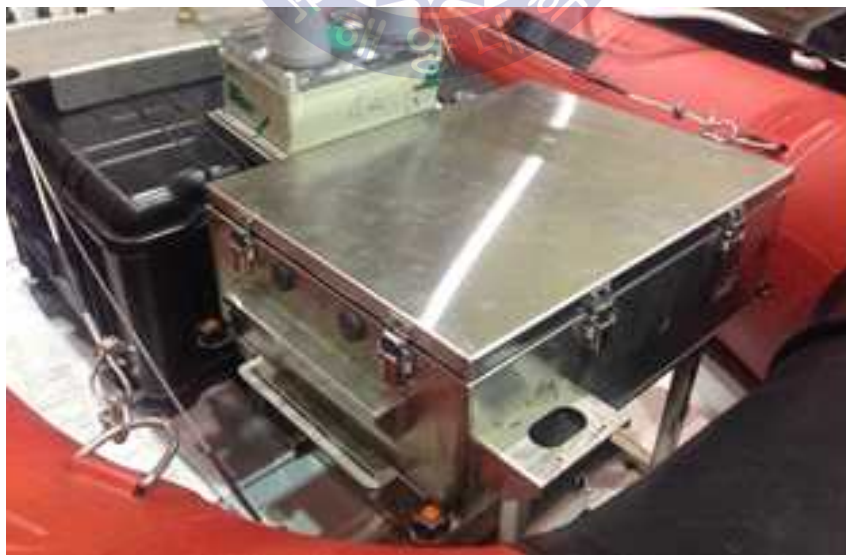
Fig 4.36 Unmanned Surface Vehicle control system installed
