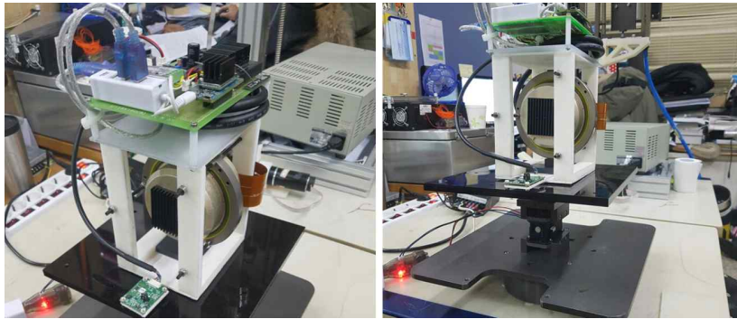
Fig 4.14 ARS test H/W(left) & rotating table(right)
