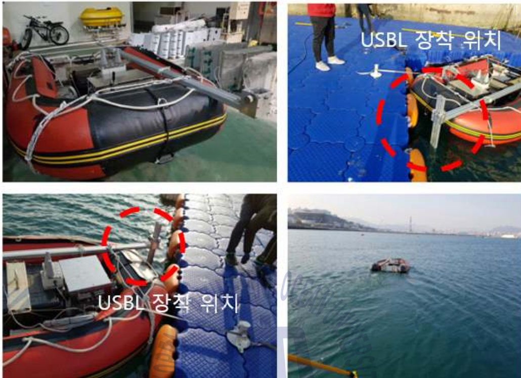
Fig 4.38 USBL mounted on Unmanned Surface Vehicle
