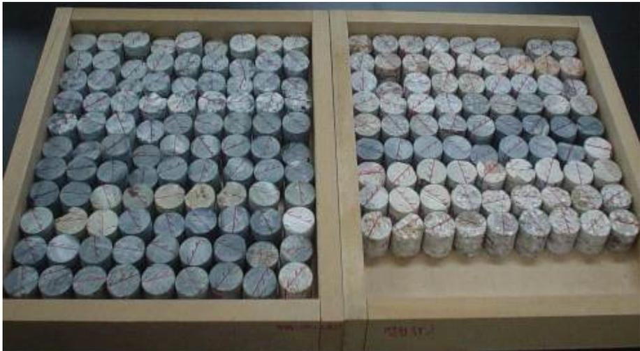
Fig. 3.4 Photograph of samples for magnetic susceptibility tests
