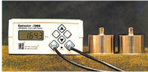
Fig. 3.12 Measurement apparatus of seismic velocity
