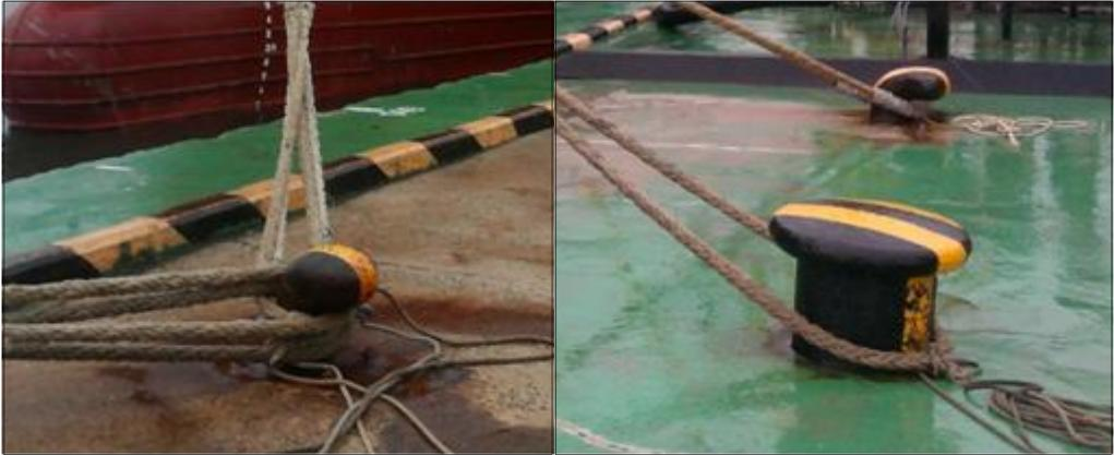
Fig. 44 Using environment of mooring post and bollard
