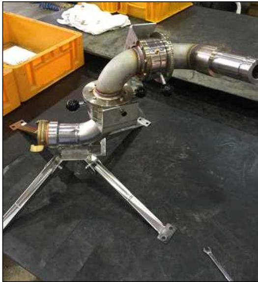
**Fig. 107** 1st Prototype of Mobile Water Monitor
