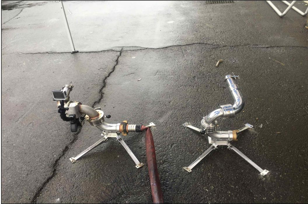
Fig. 108 Setting Prototypes for Horizontal Throw Length Test
