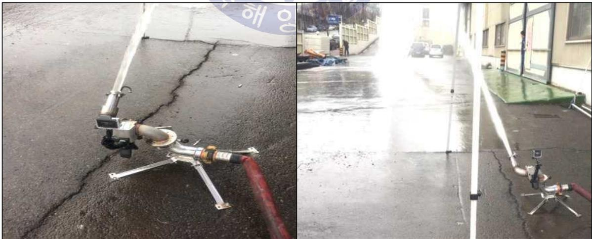
Fig. 112 Performance Test of 1st Prototype Mobile Water Monitor
