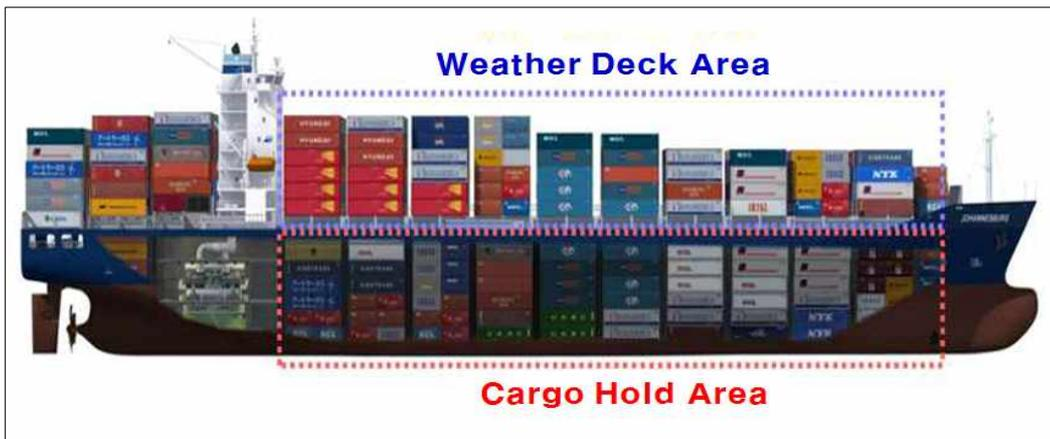
Fig. 5 Cargo Area of Container Ship
