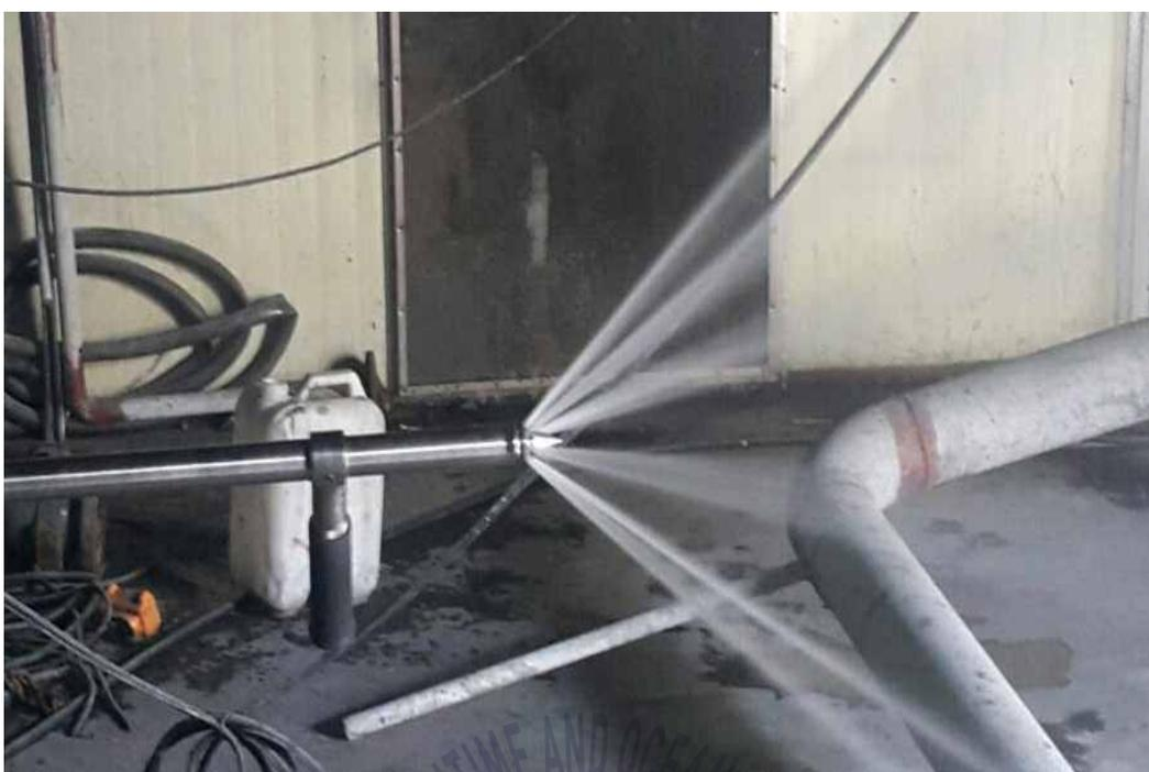
Fig. 72 Picture of Flow Test For Water Mist Lance Nozzle
