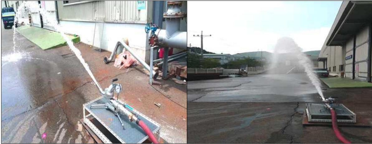
Fig. 129 Performance Test of Final Prototype Mobile Water Monitor
