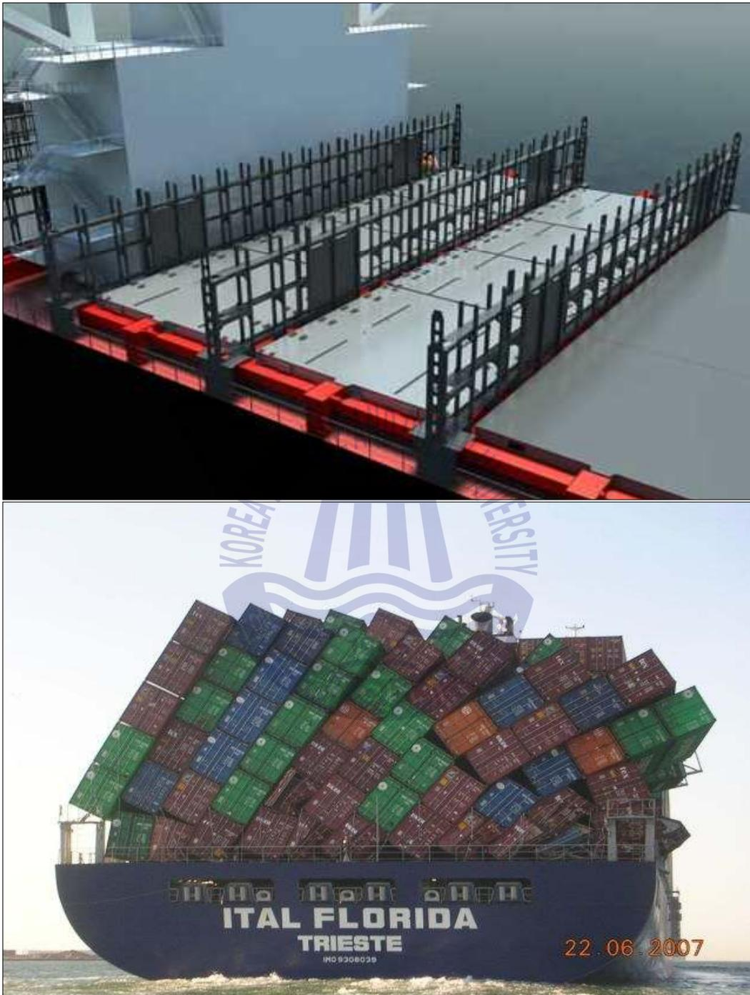
Fig. 131 Picture of Lashing Bridge(up, cargotec) and Accident(down, in.printerest.com)
