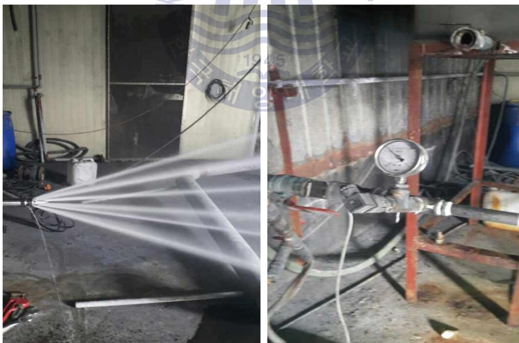
Fig. 73 Picture of Flow Test For Water Mist Lance Nozzle
