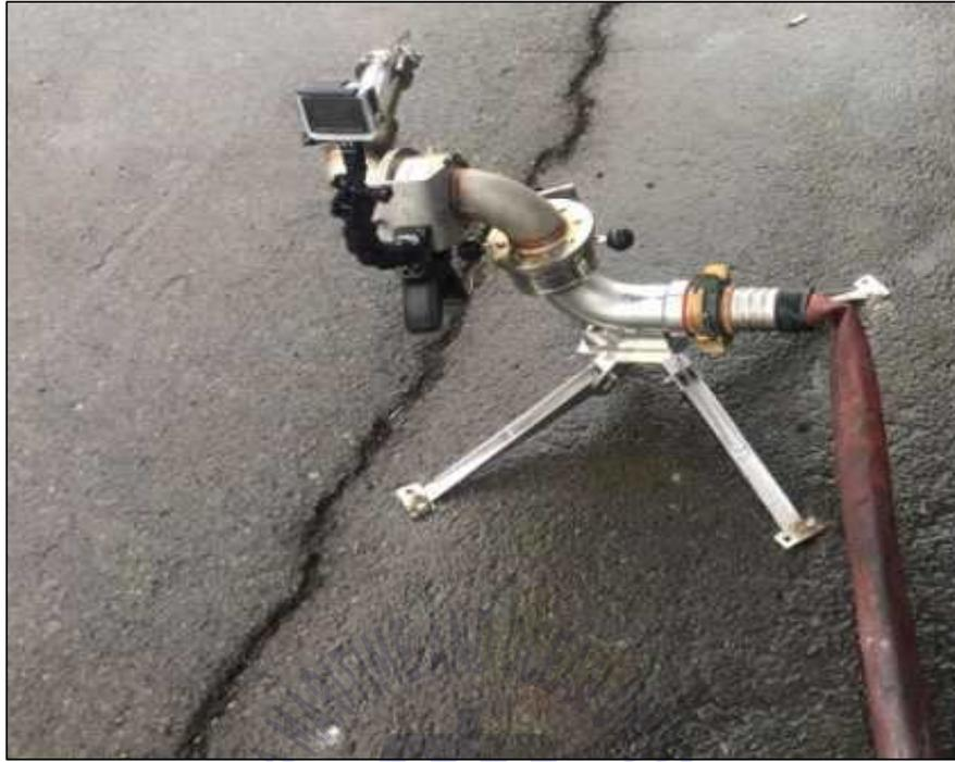
Fig. 111 Setting of 1st Prototype Mobile Water Monitor
