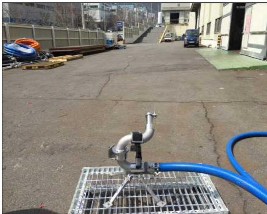
Fig. 113 Setting of 2nd Prototype Mobile Water Monitor
