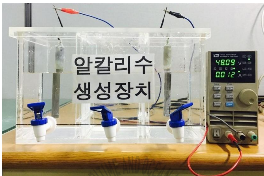
Fig. 18 Generating equipment for Alkaline water
