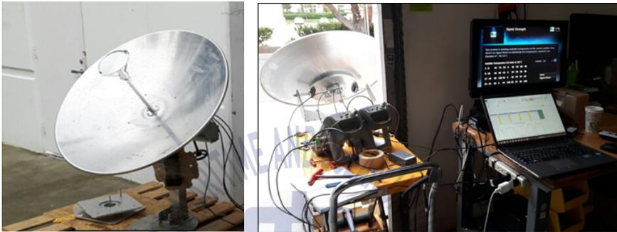
Fig. 39 Test configuration for signal quality measurement
