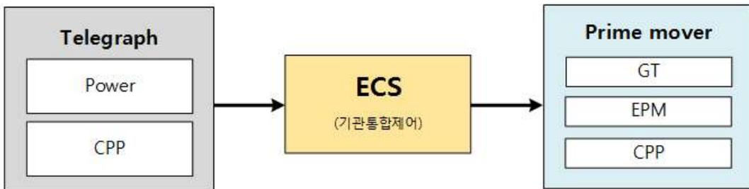
**Fig. 36** ECS Control flow
