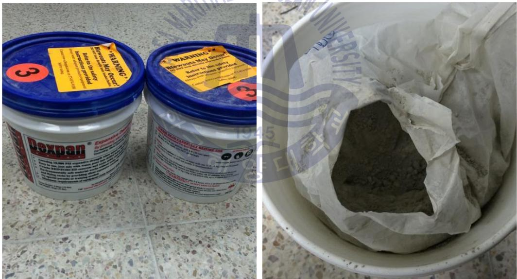
Fig. 4-1 Soundless Chemical Demolition Agent (Dexpan)
