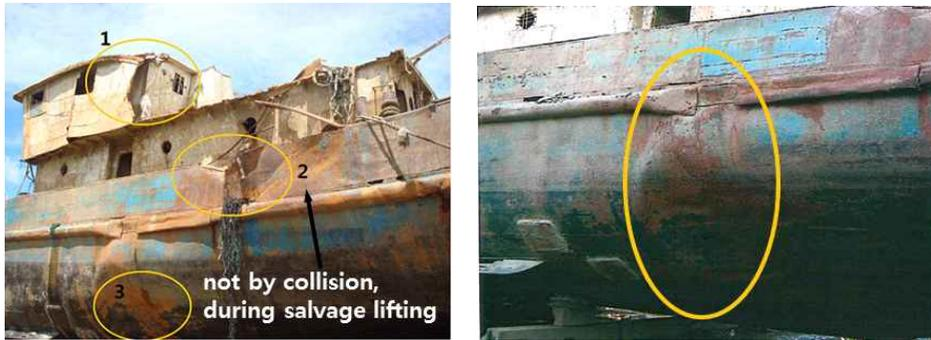
Fig. 10 Collision damage configuration of struck fishing vessel
