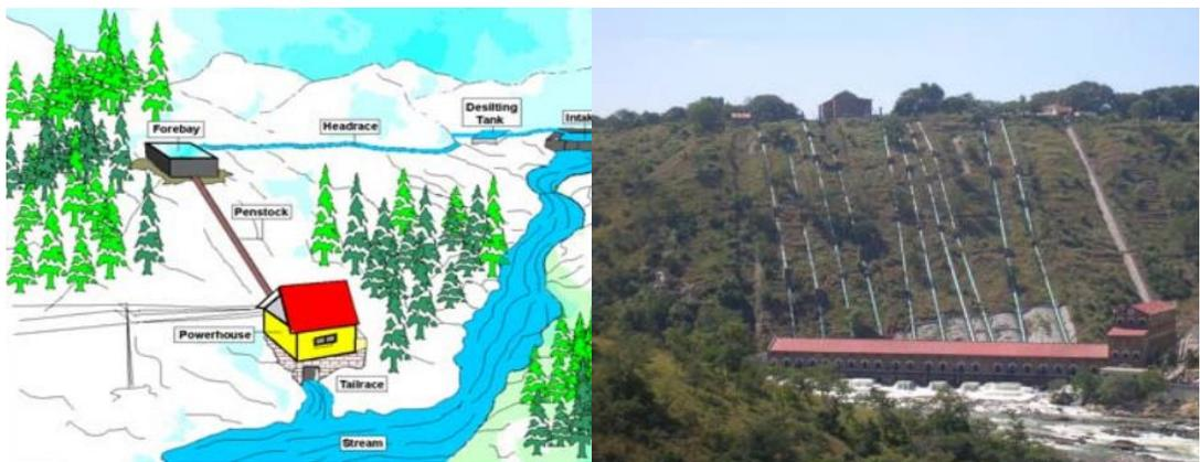
Figure 1.2 River power plant schema
