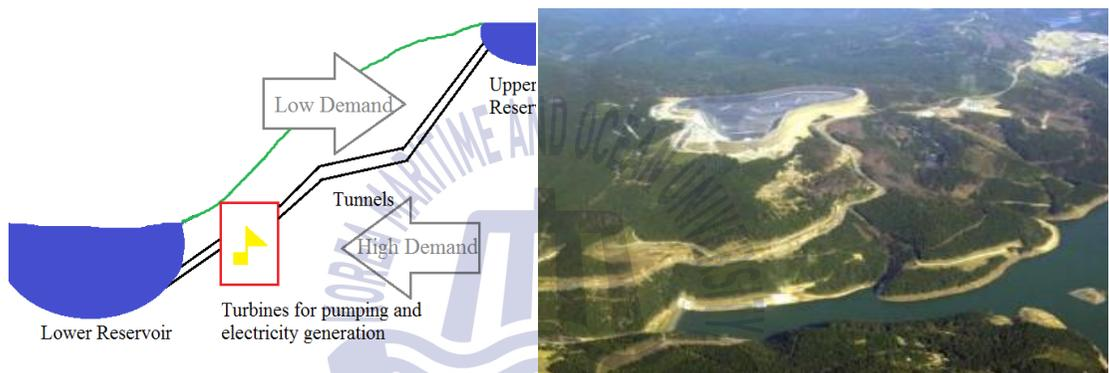
Figure 1.3 Storage hydropower plant
