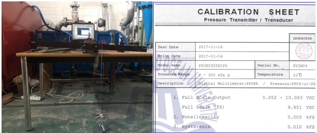
Figure 4.7 Pressure and torque transducer Calibration sheet
