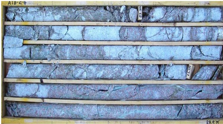
Fig. 3.12 Collapse tunnel type with granite inclusions
