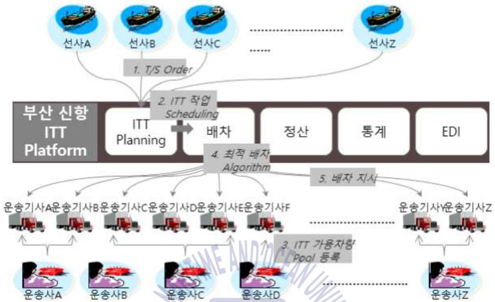
Fig. 4-7 ITT Platform 배차 Process
