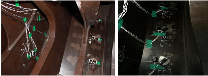
Fig. 3-5 Strain gauge sensors installed on the shell plating and at the transverse frame
