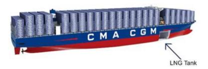
Fig. 2-14 CMA CGM gas-fueled newbuilds with GTT membrane tank (GTT, 2017)
