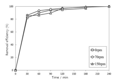
Fig. 20 The effect of agitation speed on the precipitation behavior of Cu ([Au]=40mg/L, [Cu]=430mg/L, 0.3% sodium hypochlorite, pH 10-11, Temperature=25℃, 240min)
