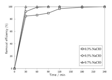
Fig. 18 The effect on the amount of sodium hypochlorite on the precipitation behavior of Cu ([Au]=40mg/L, [Cu]=430mg/L, pH 10-11, Agitation speed=150rpm, Temperature=25℃, 240min)
