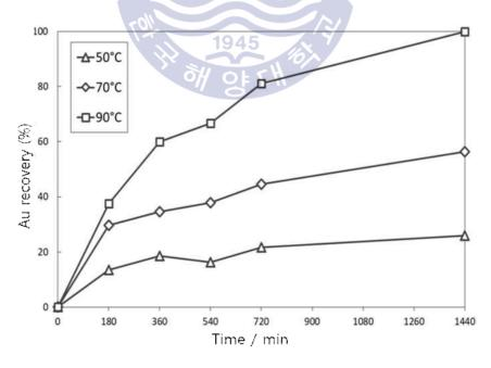
Fig. 13 The effect of temperature on the adsorption behavior of Au ([Au]=100mg/L, 0.1M NaCl, pH 6-8, 0.3g magnetite, Agitation speed=150rpm, 1440min)
