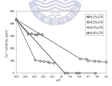
**Fig. 25** Change in solubility of copper with decreasing pH under different cyanide concentration conditions
