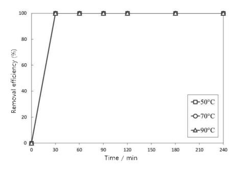
**Fig. 22** The effect of temperature on the precipitation behavior of Cu ([Au]=40mg/L, [Cu]=430mg/L, 0.3% sodium hypochlorite, pH 10-11, Agitation speed=150rpm, 240min)
