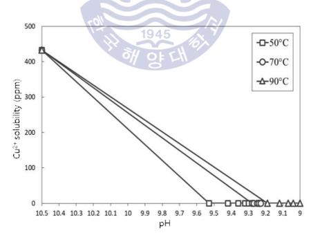
Fig. 23 Change in solubility of copper with decreasing pH under different temperature conditions
