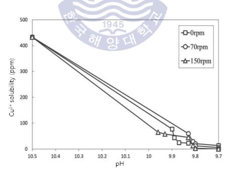
Fig. 21 Change in solubility of copper with decreasing pH under different agitation speed conditions
