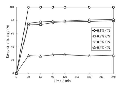
Fig. 24 The effect of cyanide concentration on the precipitation behavior of Cu ([Au]=40mg/L, [Cu]=430mg/L, 0.3% sodium hypochlorite, pH 10-11, Agitation speed=150rpm, 240min)
