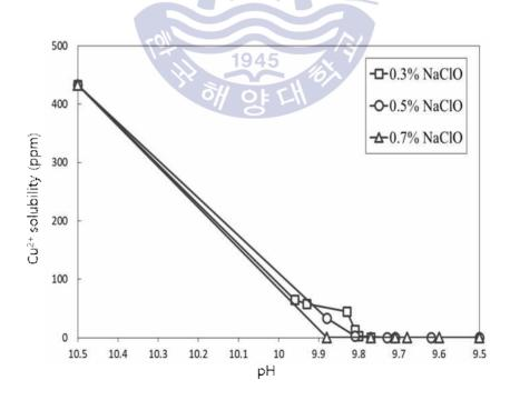
Fig. 19 Change in solubility of copper with decreasing pH under different amounts of sodium hypochlorite
