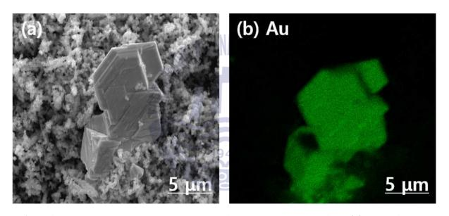
Fig. 16 SEM and EDS elemental mapping of the magnetite: (a) SEM image, (b) Elemental mapping of Au
