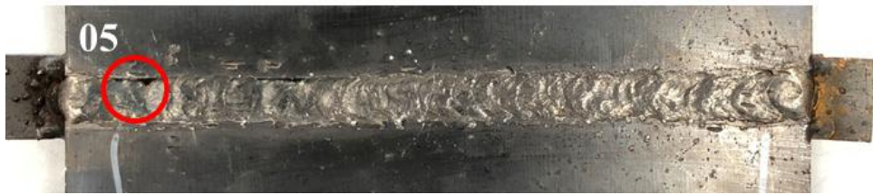
Fig. 18 Front of failure specimen 05
