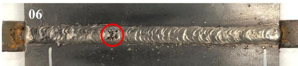
Fig. 21 Front of failure specimen 06
