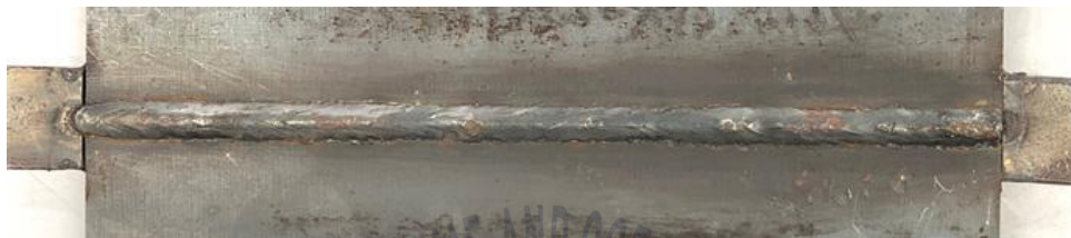
Fig. 19 Back side of failure specimen 05
