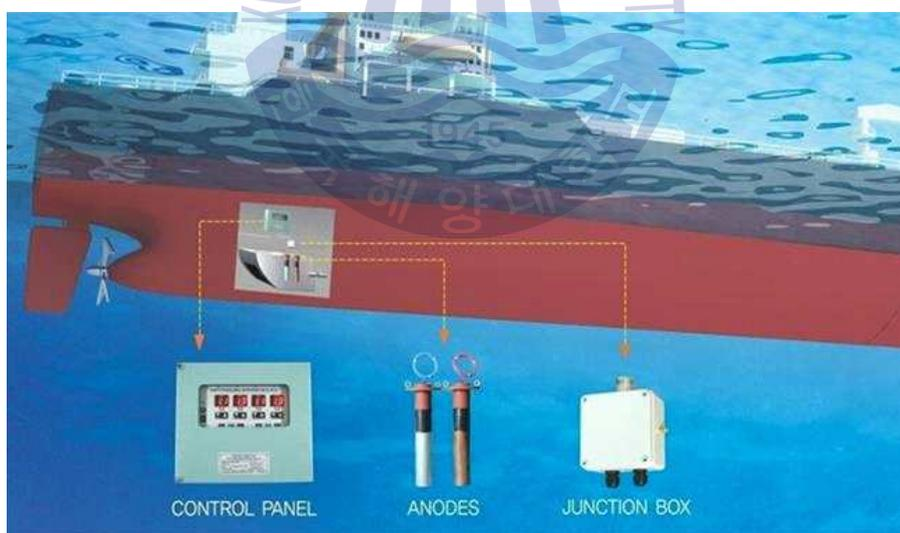
Fig 2.33 Schematic drawing of the MGPS
