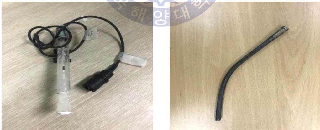
Fig 3.8 Auxiliary test apparatus for cathodic protection in the cistern, (a): Silver-silver/chlorine electrode, (b): Rod type MMO anode
