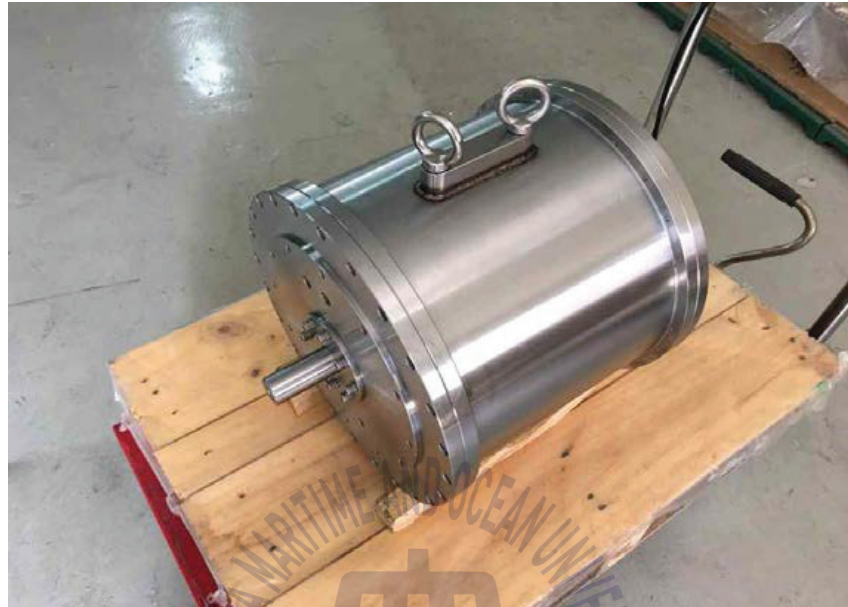
(a) Test model with air-gap 2 mm
