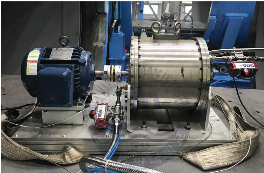
Fig 5.20 Installation of test sample for rotational speed condition test
