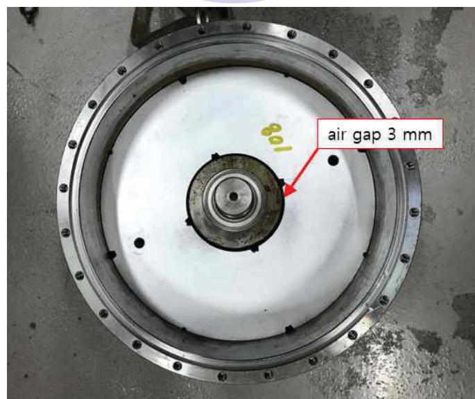
Fig 5.14 Test sample with air-gap 3 mm
