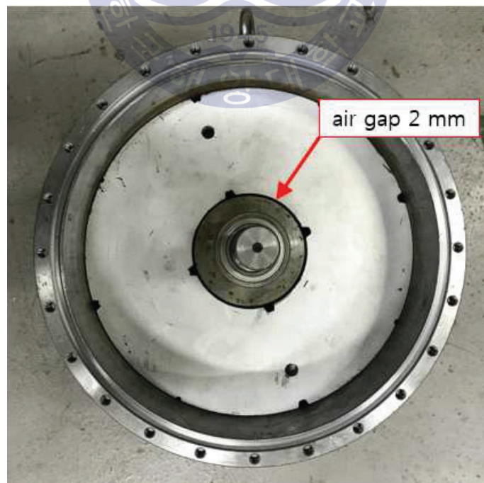
(b) Internal construction for test model
