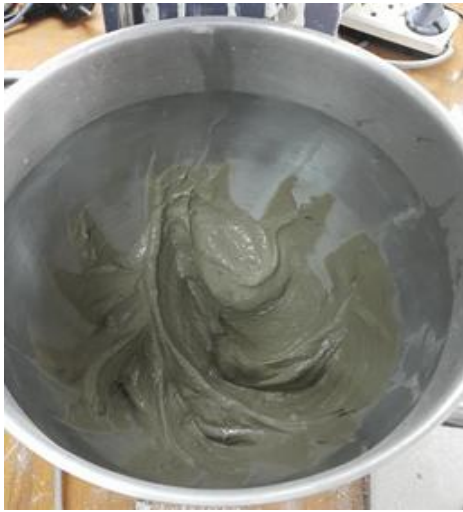
(a) Mixing cement slurry
