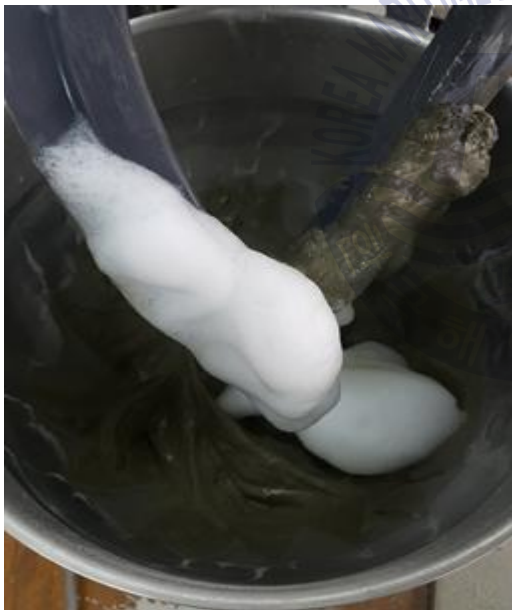
(c) Mixing foam and cement slurry
