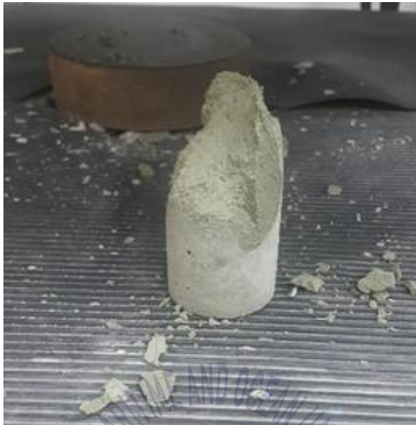
Fig. 3.6 Failure shape of specimen
