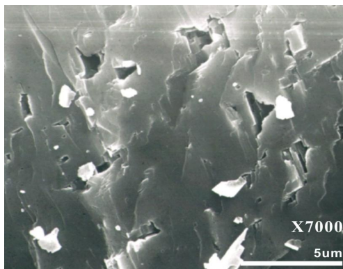
(a) Slight weathered feldspar
