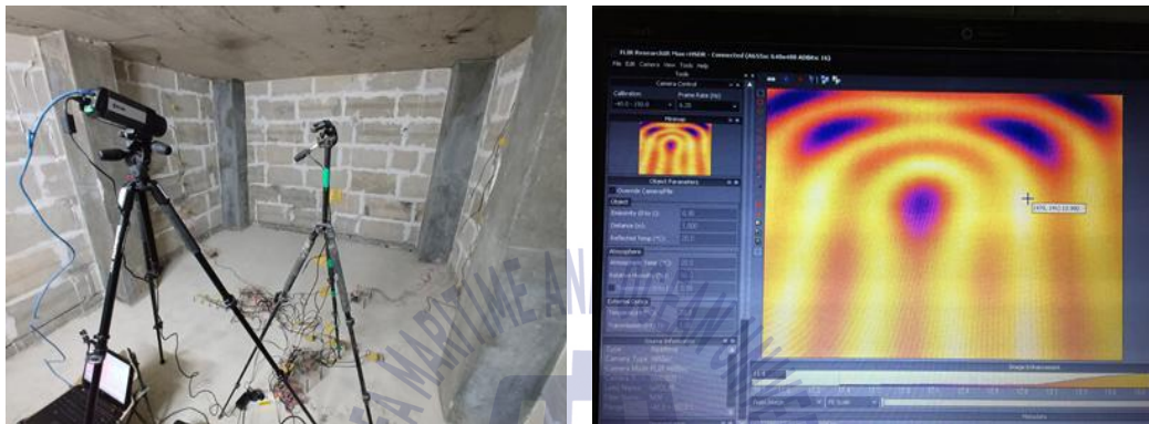
(a) Thermal imaging camera(FLIR A615) (b) Real-time shooting scenes(FLIR Tools)
