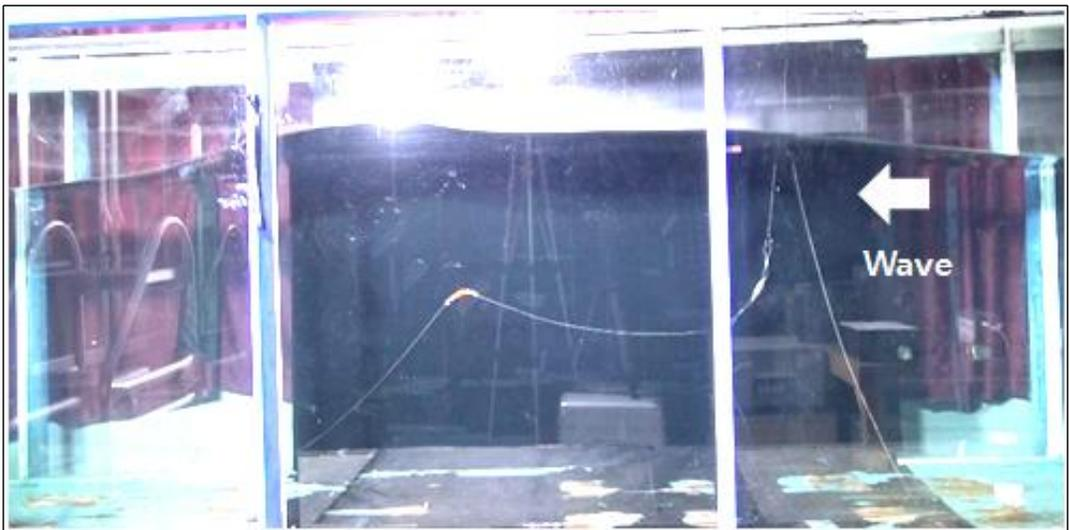
**Fig. 4.56** Behavior characteristics of dynamic cable (LC1, After wave generation)
