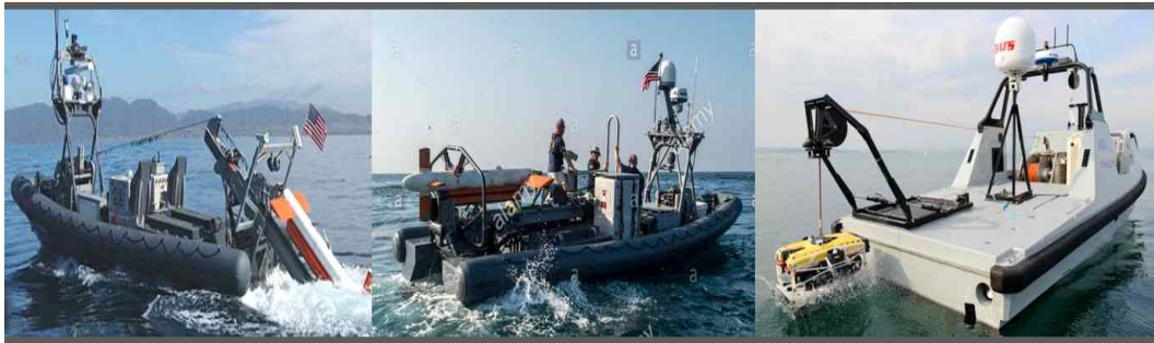
Fig. 5-2 Launch & Recovery System
