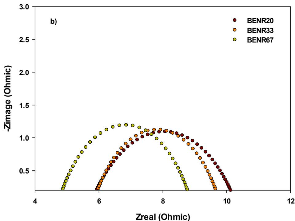
Fig. 6.5. Electrochemical analysis for the bulk solution of BENRs: a) CV b) Nyquist plot for the EIS data
