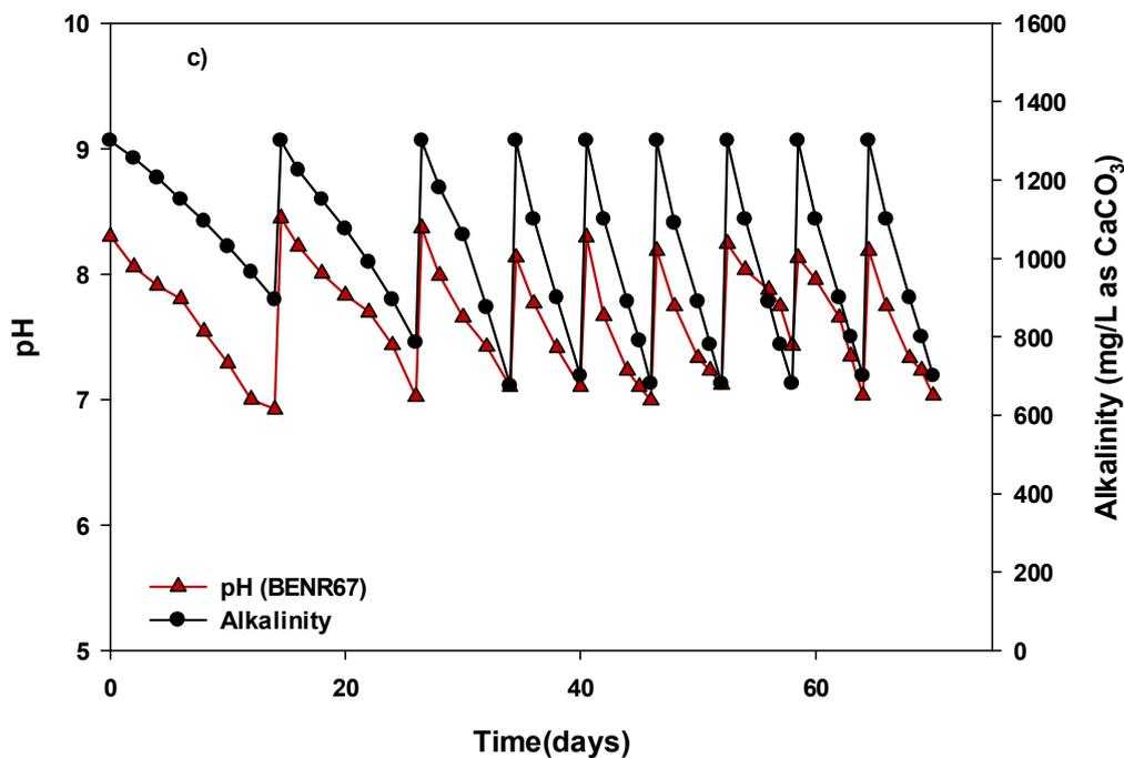
Fig. 6.3 Changes in pH and alkalinity in bioelectrochemical nitrogen removal reactor
