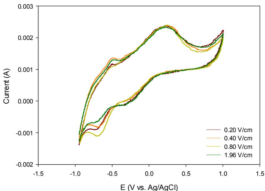
Fig 7.3. Cyclic voltammogram in the bulk solution of bioelectrochemical reactors
