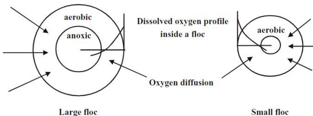
Fig. 2.3 Schematic of oxygen concentration profile within a microbial floc
