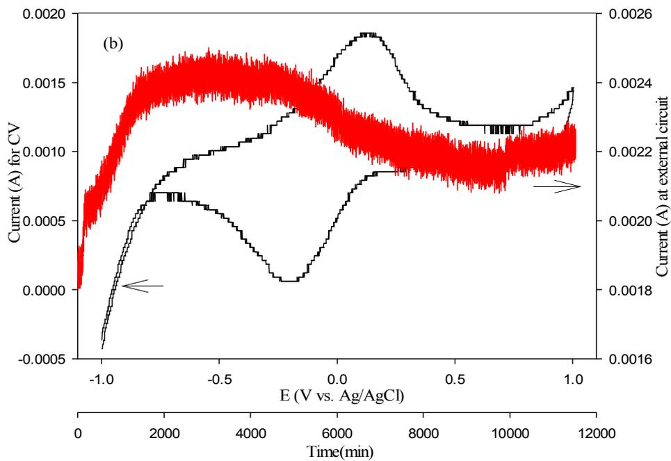
Fig.4.3 (a) Changes in pH and alkalinity and (b) cyclic voltammogram (black) and electric current (red) during the 6th batch cycle
