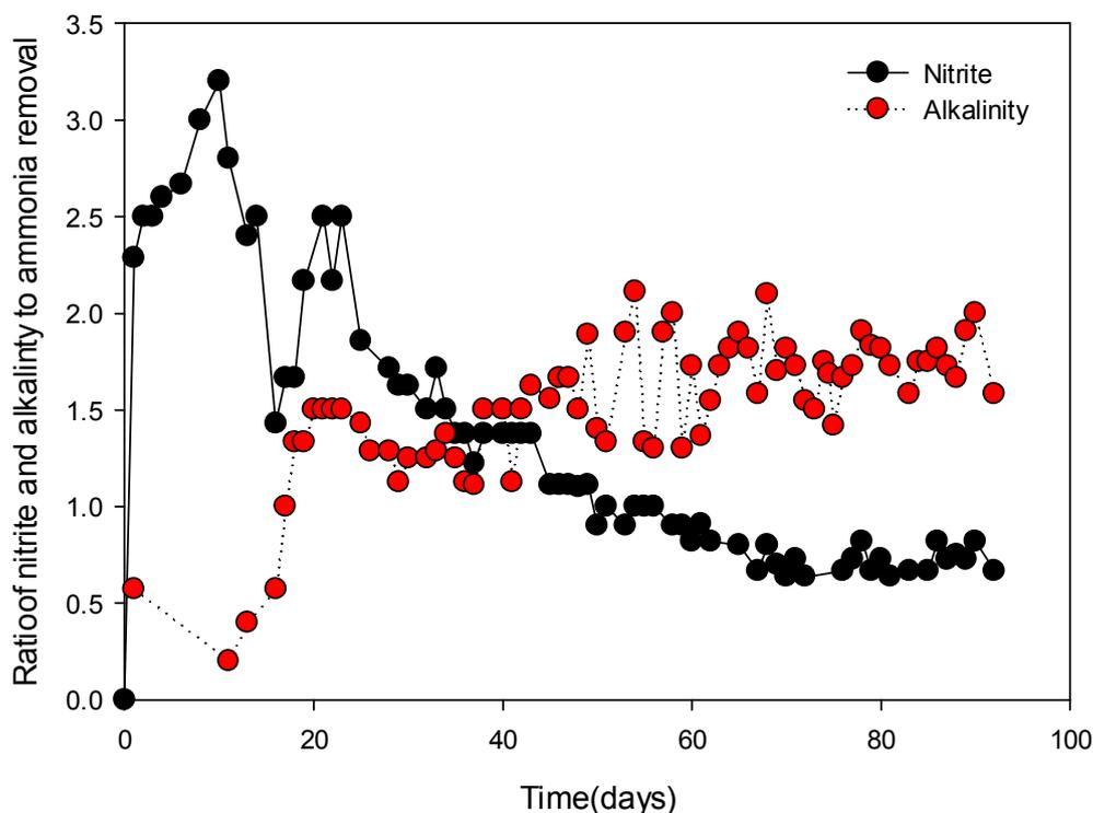
Fig.4.5 Changes of nitrite and alkalinity ratio for ammonium nitrogen removal
