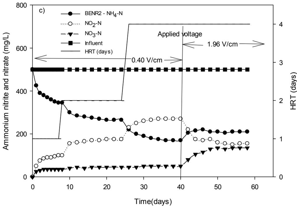
Fig 7.1. Effluent profiles in a) Control, b) BENR1 and c) BENR2
