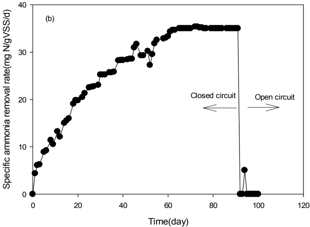
Fig.3.4 Changes in (a) VSS and (b) specific ammonia removal rate with operation time in bioelectrochemical reactor.
