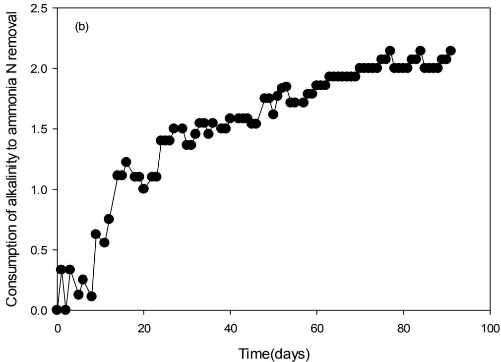
Fig.3.3 (a) Nitrite N and (b) alkalinity consumptions relative to the removal of ammonia N with operation time of the bioelectrochemical batch reactor.
