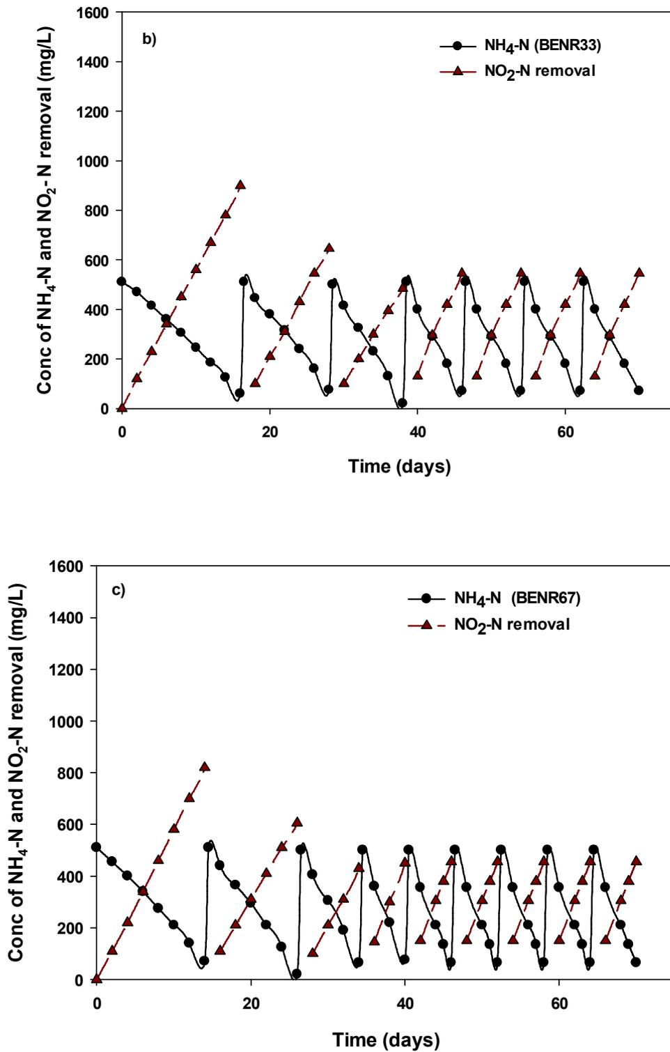
Fig.6.2 Changes in ammonium and nitrite nitrogen in bioelectrochemical nitrogen removal reactor: a) BENR20, b) BENR33 and c) BENR67
