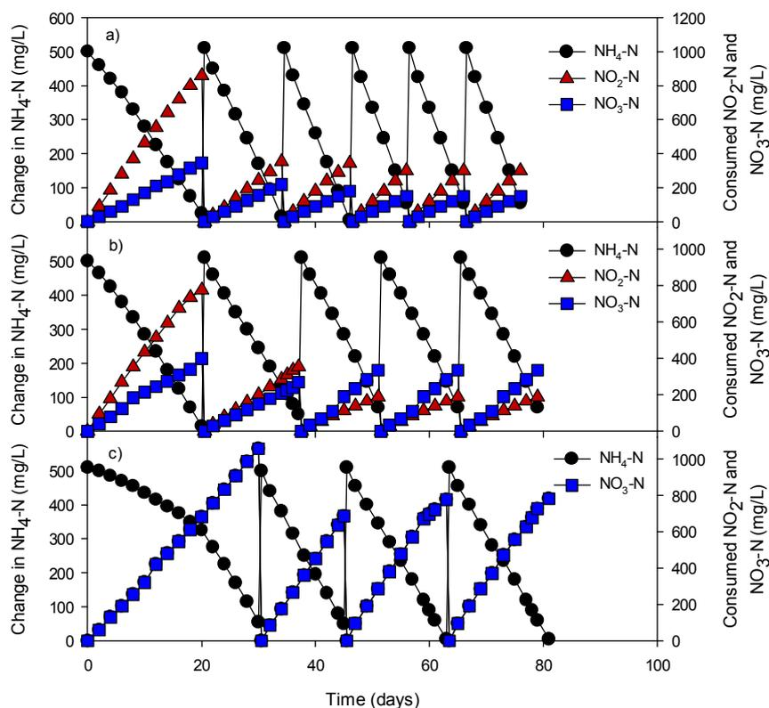
Fig. 5.2. Concentration changes in ammonium and consumed nitrite and nitrate. a) BENR1, b) BENR2, and c) BENR3
