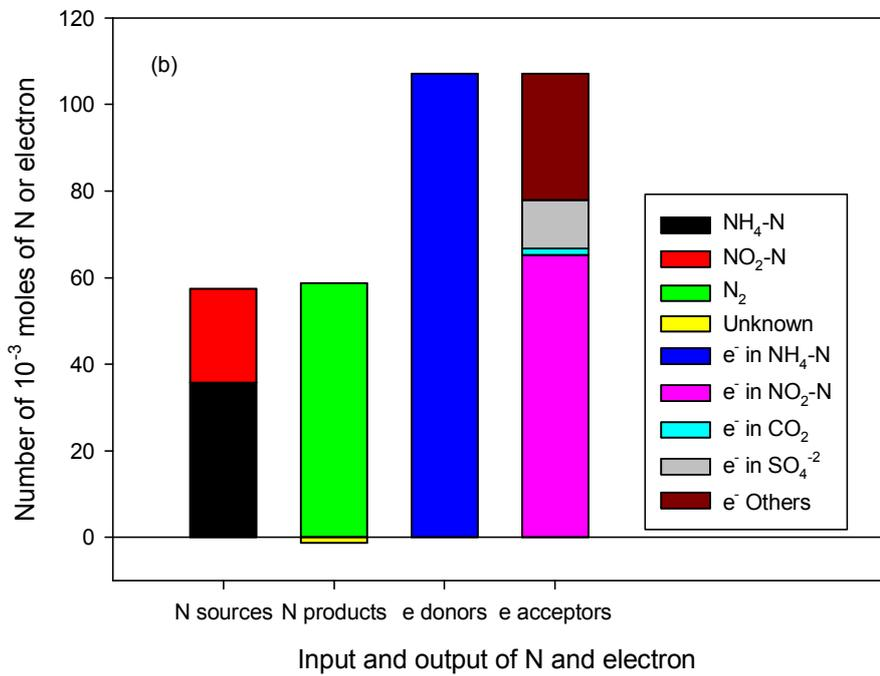
Fig.4.4 (a) Cumulative biogas production in the bioelectrochemical reactor and (b) nitrogen and electron balance during the 6th batch cycle
