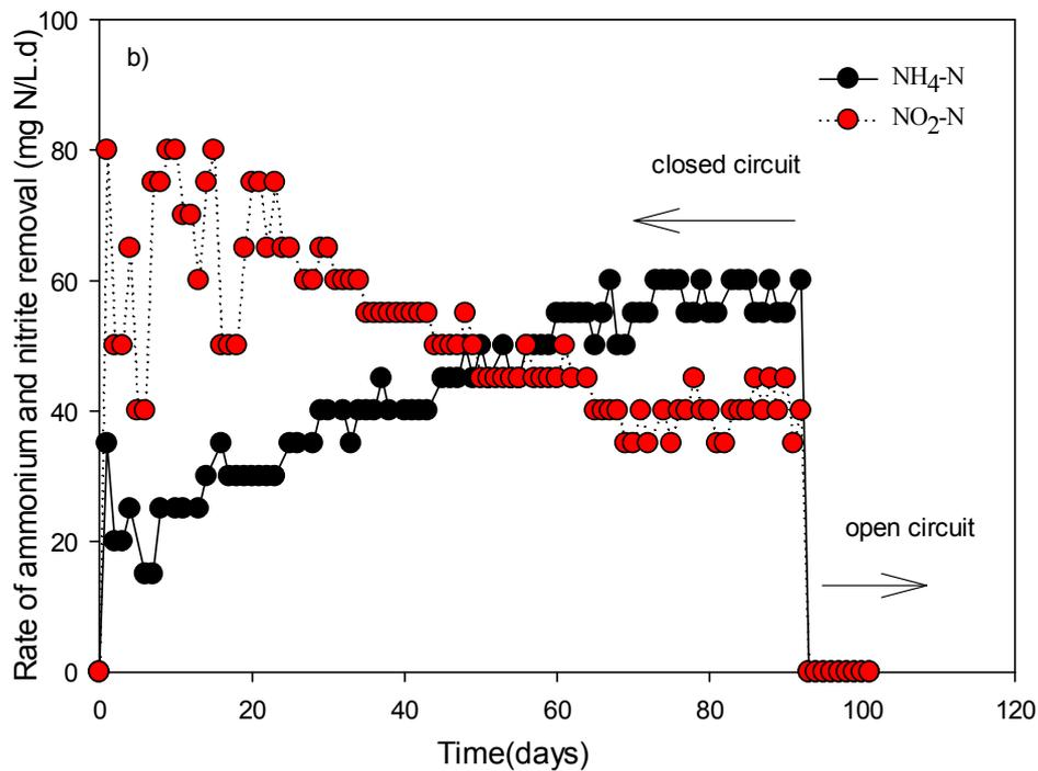
Fig.4.1 (a) Changes in ammonium and nitrite nitrogen and (b) their removal rates in bioelectrochemical batch reactor
