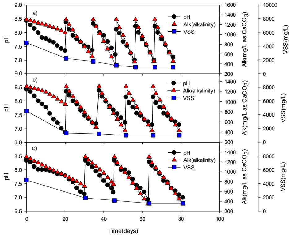
Fig. 5.3. Changes in pH, alkalinity, and VSS concentrations. a) BENR1, b) BENR2, and c) BENR3
