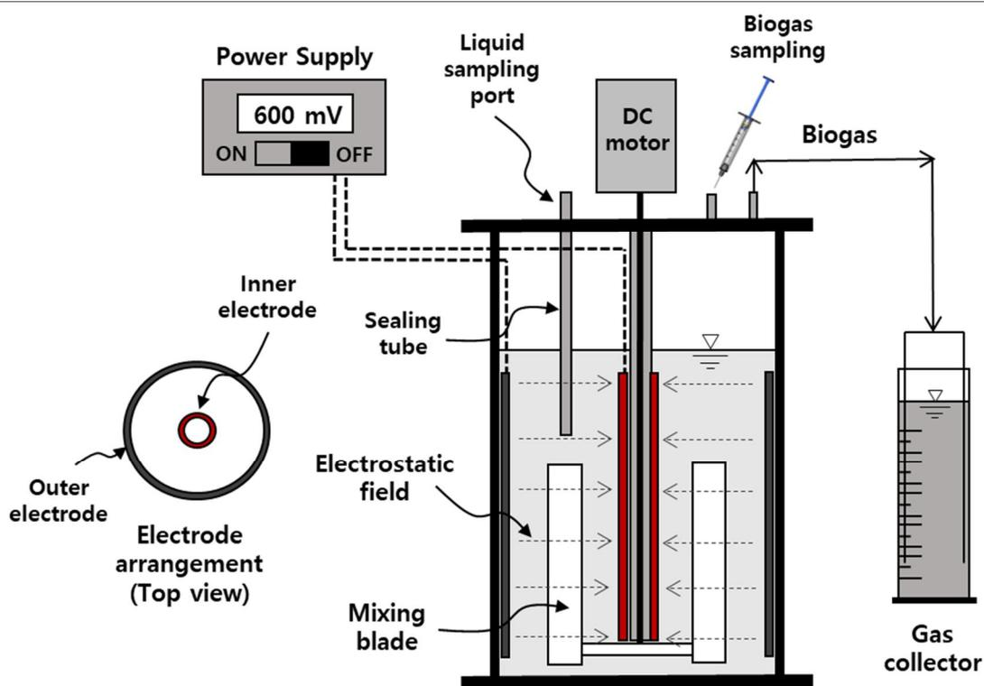
Fig.6.1 Schematic diagram of bioelectrochemical nitrogen removal reactor exposed to the electrostatic field.
