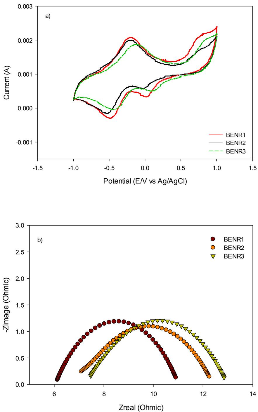
Fig. 5.4. Electrochemical analysis for the bulk solution of BENRs. a) Cyclic voltammogram, b) Nyquist plot for the EIS data
