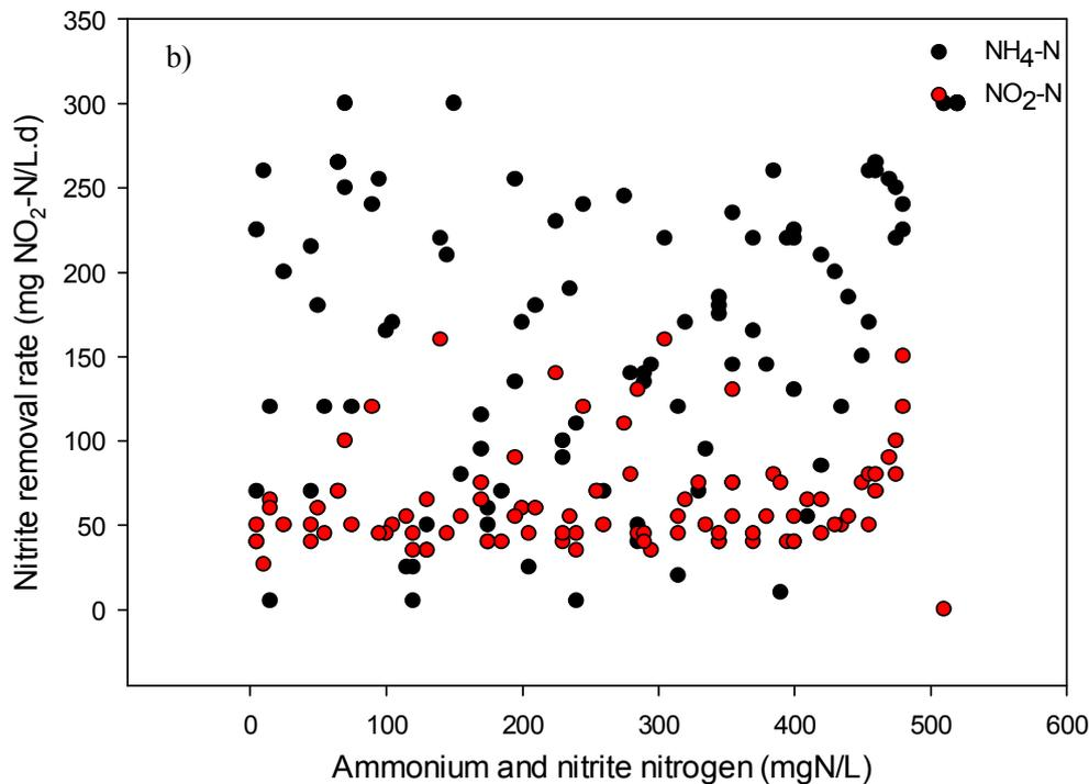
Fig.4.2 (a) VSS decreases in bioelectrochemical reactor and b) dependence of nitrite removal rate on the ammonium and nitrite nitrogen
