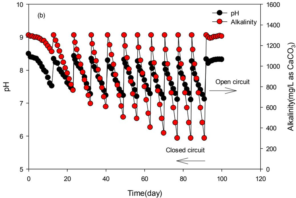
Fig.3.1 Changes of (a)  $\text{NH}_4\text{-N}$  and  $\text{NO}_2\text{-N}$  and (b) pH and alkalinity in bioelectrochemical reactor during batch operation
