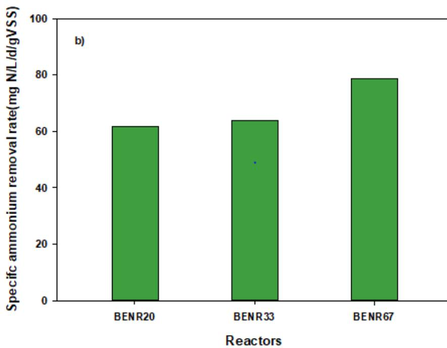
Fig.6.4 a) VSS levels retained and b) specific ammonium removal rate in BENR at steady state, depending on the electrostatic field
