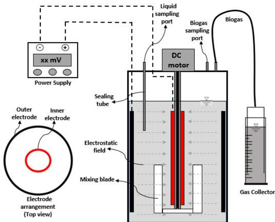
Fig. 5.1. Schematic diagram of bioelectrochemical nitrogen removal reactor
