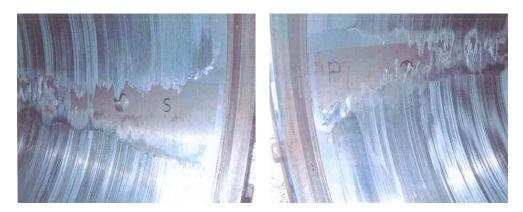
Fig. 2.1 An example of the damage of after stern tube bearing
