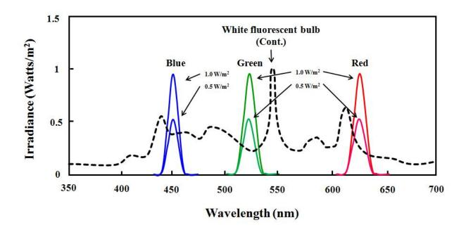
**Fig. 6.** Spectral profiles of red, green, and blue light emitting diodes (LEDs) and white fluorescent bulb (control) used in this study. Different light intensities (0.5 and 1.0 W/m<sup>2</sup>) were used for each type of LED.
