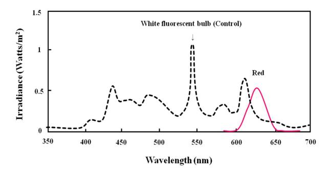
**Fig. 14.** Spectral profiles of red light emitting diodes (LEDs) and white fluorescent bulb (Cont.) used in this study. The light intensities (0.5 W/m²) were used for each type of LED.
