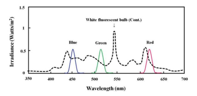
**Fig. 1.** Spectral profiles of red, green, and blue light-emitting diodes (LEDs) and the white fluorescent bulb (Cont.) used in this study. The same light intensities (0.5 W/m²)were used for each type of LED.
